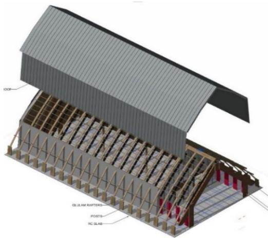
*Figure 11. a digital model of the proposed Tānewhirinaki whareniui using mīmirū portals. The geometry of this proposal established the geometry of the portals used in this research:*
