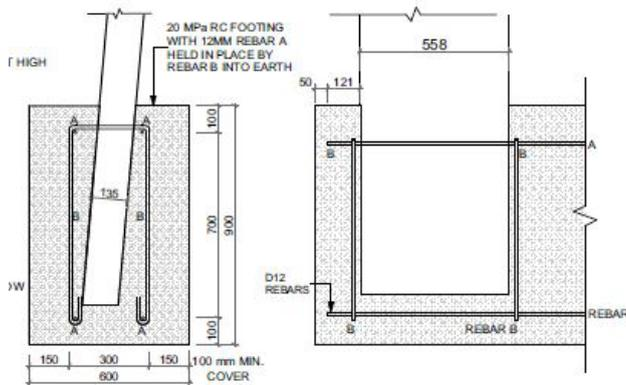
Figure 4. The 900mm deep reinforced concrete footings were dug by hand.
