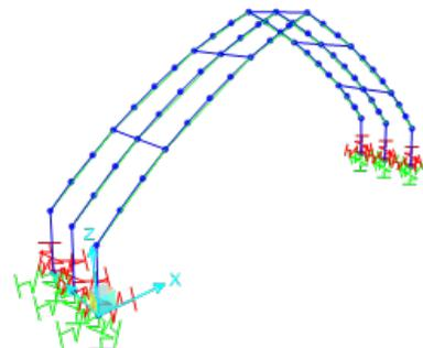
*Figure 10. Preliminary FEM SAP2000 Isometric showing inclusion of Rotational Springs at Foundation. Image: Sonny Vercoe*
