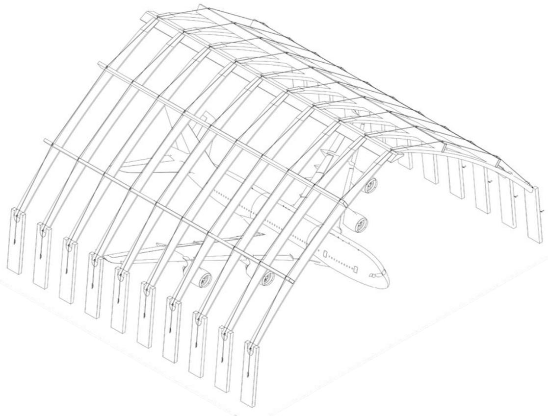
Figure 12. Proposed Mīmirū Portals used to create a UAV hangar spanning 40m+. Image: Anthony Hōete
