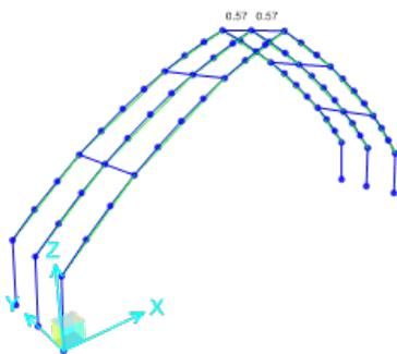
*Figure 9. Preliminary FEM SAP2000 Isometric showing Line Mass and Tendon Elements. Image: Sonny Vercoe*
