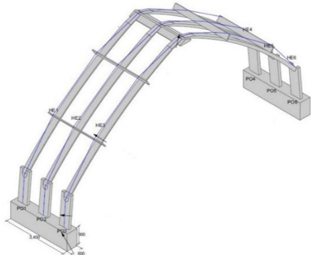
Figure 5. The full-scale prototype consisted of three portals (tāhuhu ridge beam section, six curved heke rafters, 4 kaho purlins and six poupou (inclined posts)). Image: Anthony Hōete.
