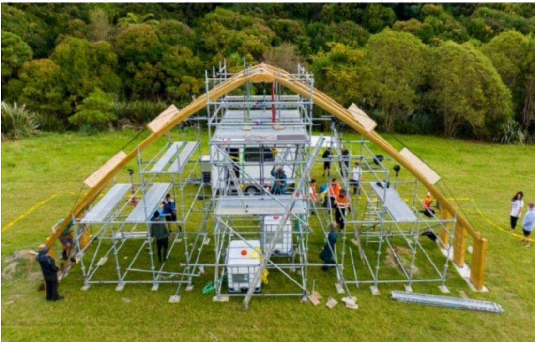
*Figure 8. Prototype portal structure showing independent scaffolding holding measuring gauges. In the bottom centre, IBCs carry the simulated vertical load. Image: Anthony Hōete.*
