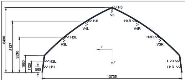
Figure 6 (above). Draw Wire Sensor placements to detect vertical and horizontal displacement. Image: Anthony Hōete.
