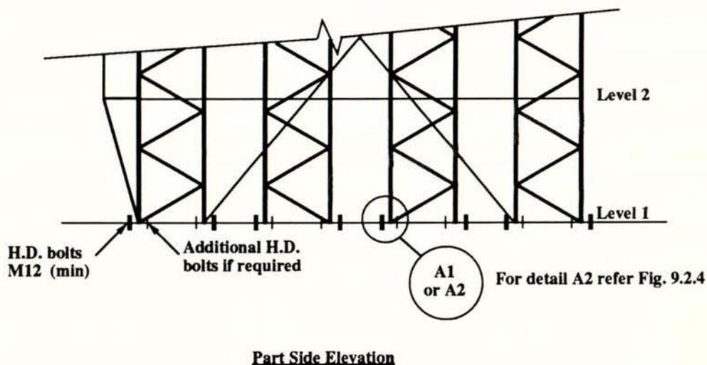
**Fig. 9.2.3 Rack Hold-Down Details - Alternative 1**
