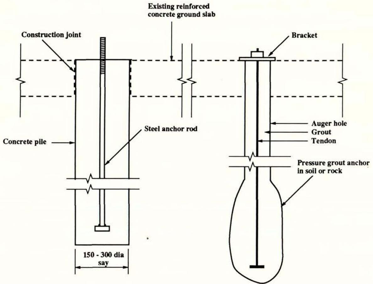
Note: Pile or anchor safe working load typically 20 - 50 kN
