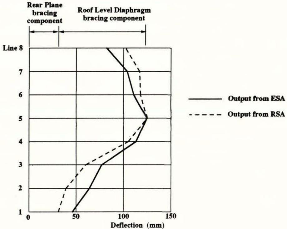
(b) Plan Deflected Shape for the Case of Pallet Rails Included in the Model and Columns Pinned Each End
