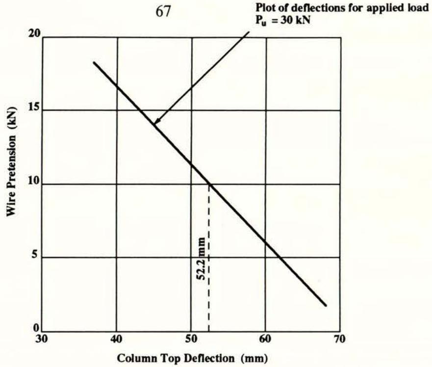
Fig. A2.2 Column Top Deflection vs Wire Pretension
