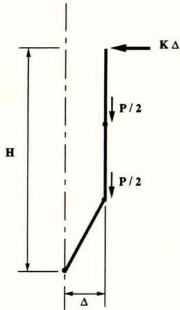
For a deflected shape as shown, and pinned ends, the equilibrium equation is :-
