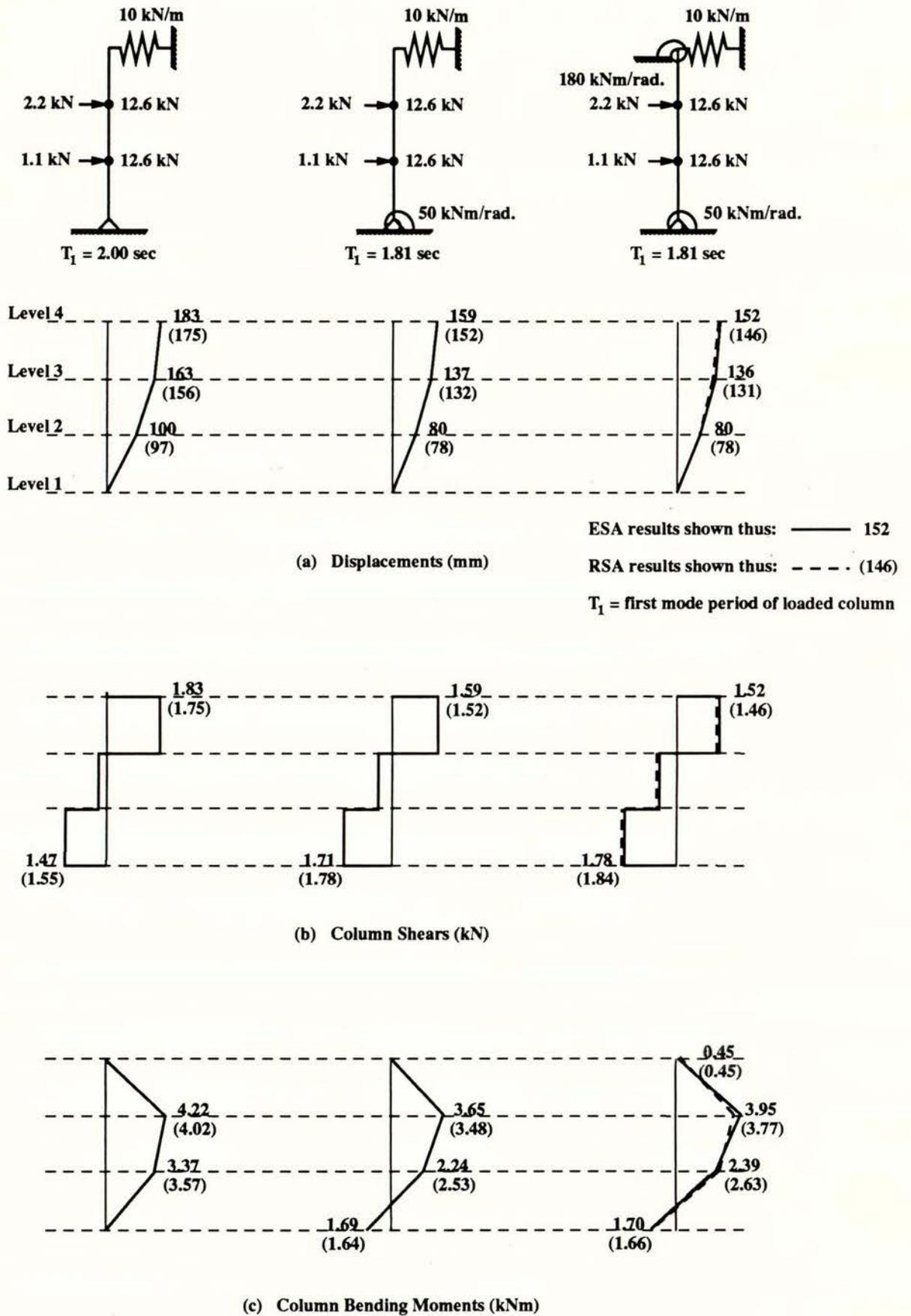
Fig. 6.3.2 COL10 Output Data For Various End Rotational Restraints and  $K_{x4} = 10 \text{ kN/m}$
