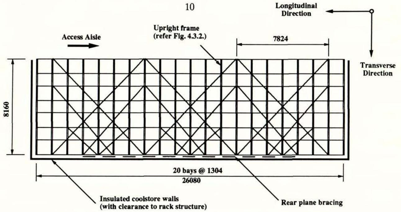
**Plan - Showing Roof Level (Top Diaphragm) Bracing**
