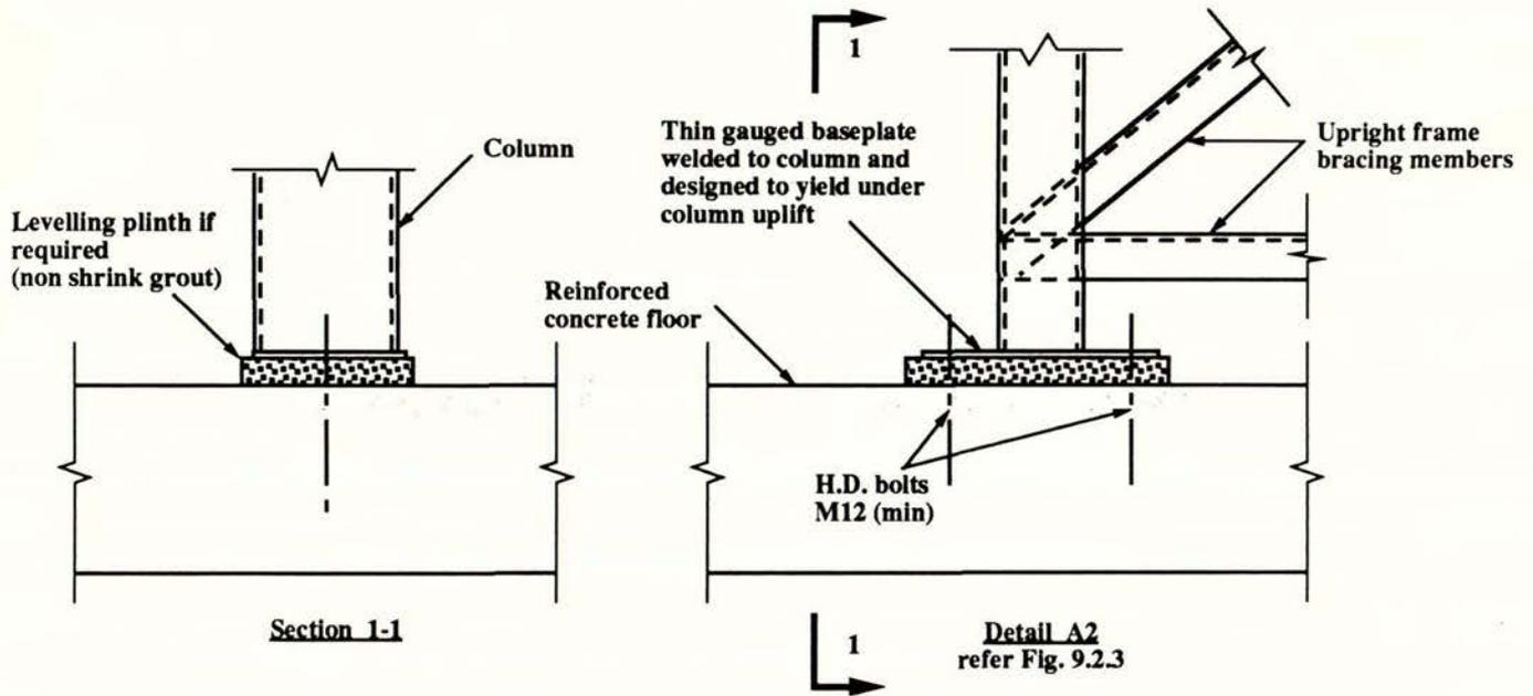
**Fig. 9.2.4 Rack Hold-Down Details - Alternative 2**
