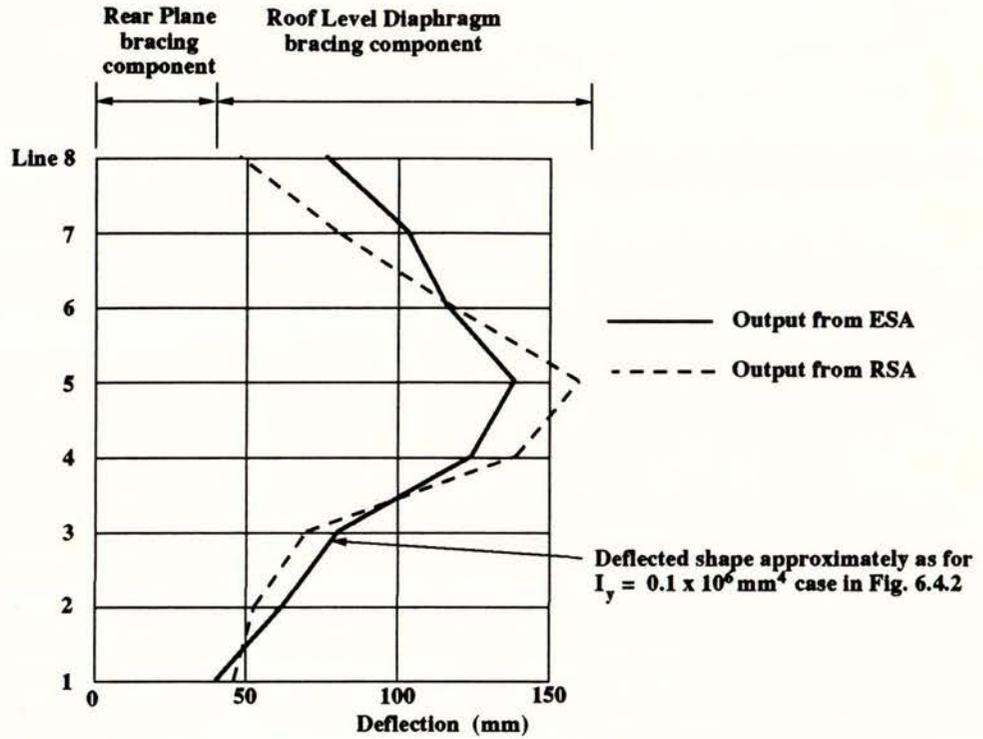
(a) Plan Deflected Shape for the Case of Pallet Rails Removed from the Model and Columns Pinned Each End
