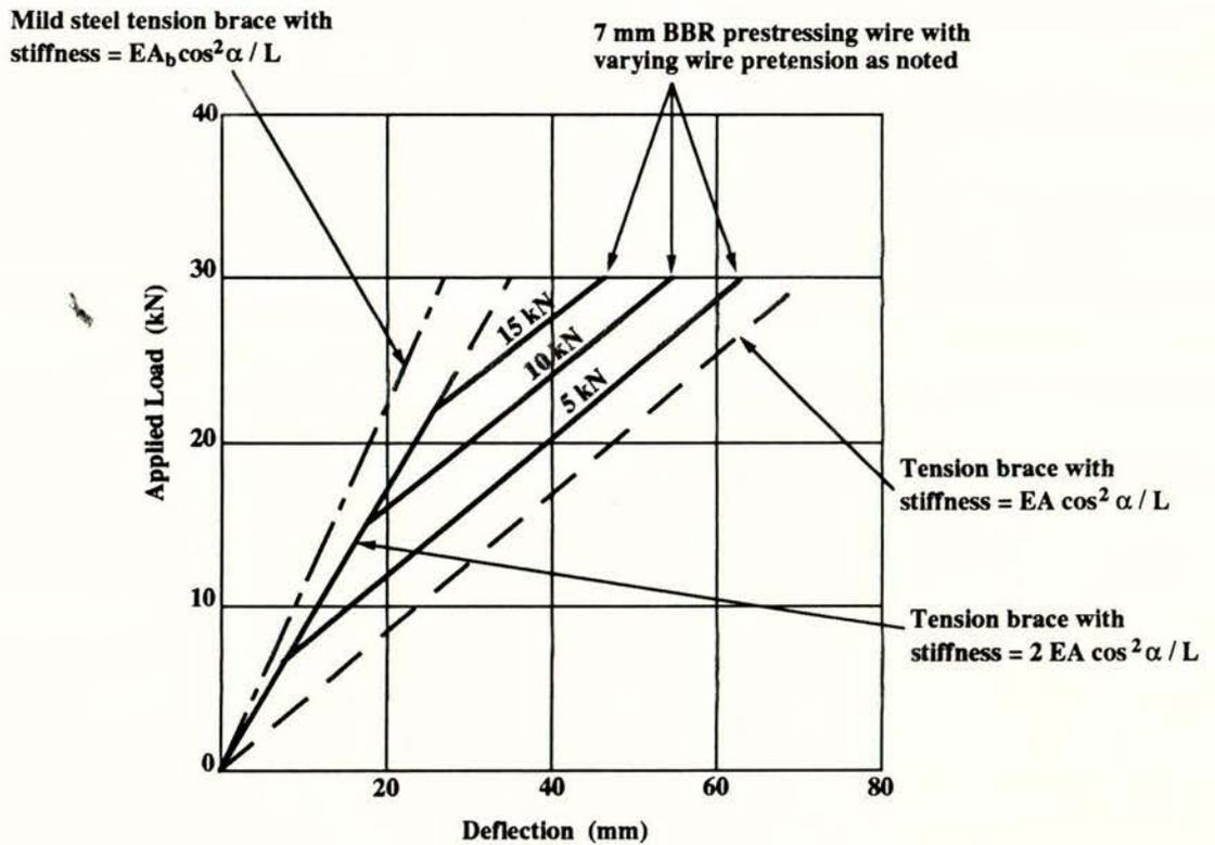
Fig. A2.3 Load-Deflection Plots For Bracing Elements Of Example A2.1
