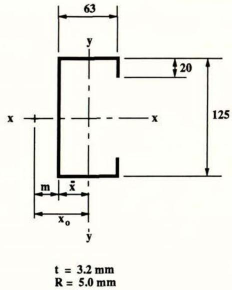
**Fig. A4.1 Column Section Properties**
