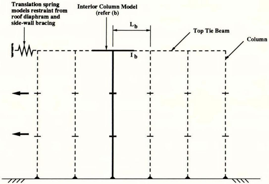
(a) Front Elevation of Drive-In Rack Loaded in the Longitudinal Direction (pallets not shown)
