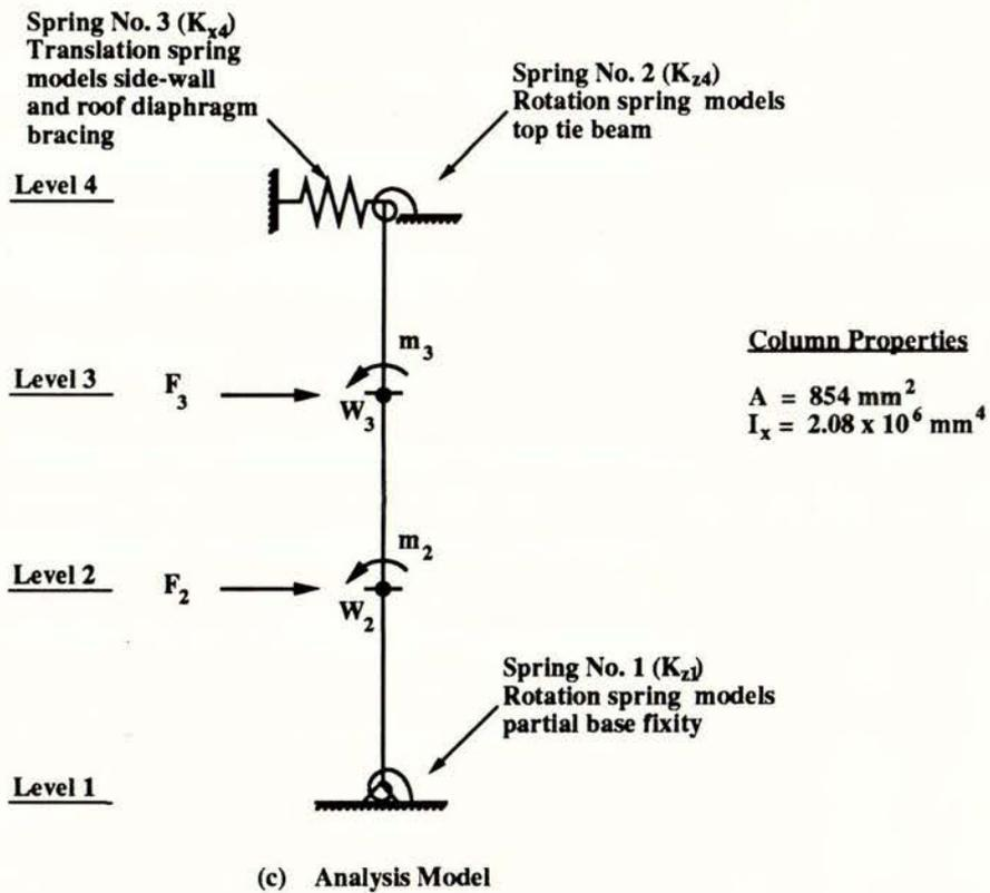
Fig. 6.3.1 Typical Interior Column Under Longitudinal Earthquake
