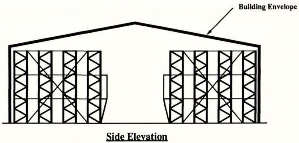
**Fig. 9.2.1 Typical Warehouse With Rack Storage**
