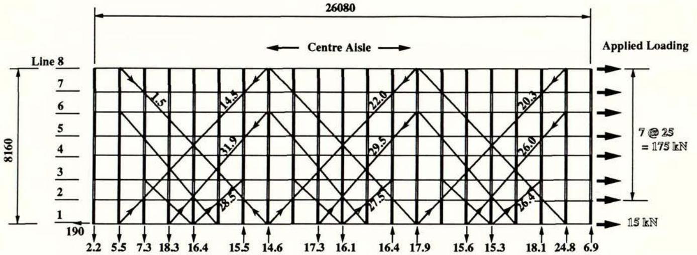
(a) Plan on Diaphragm showing Applied Loading, Bracing Loads and Reactions (kN)
