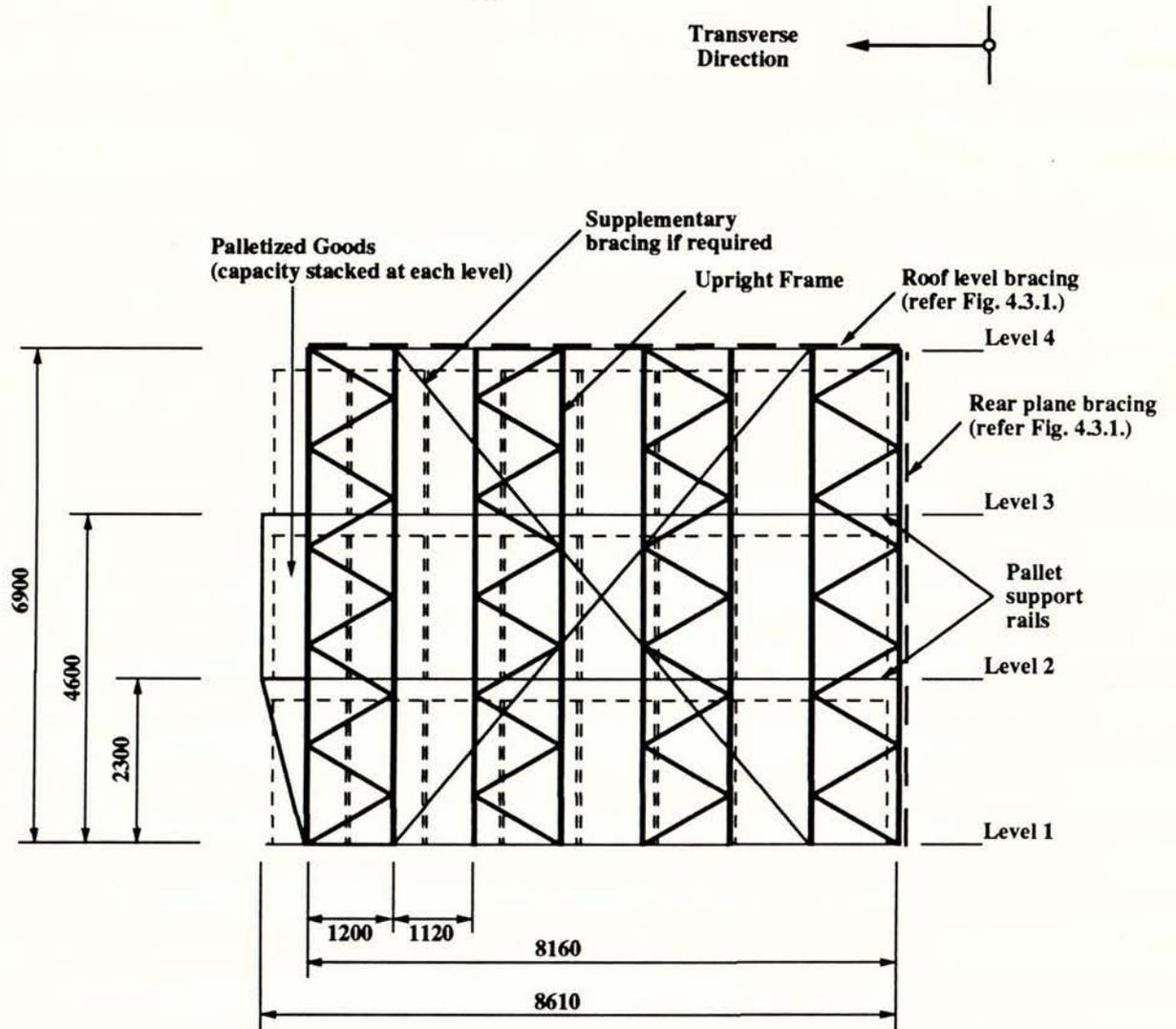
Fig. 4.3.2. Side Elevation of Drive-In Rack showing Upright Frames and Transverse Bracing
