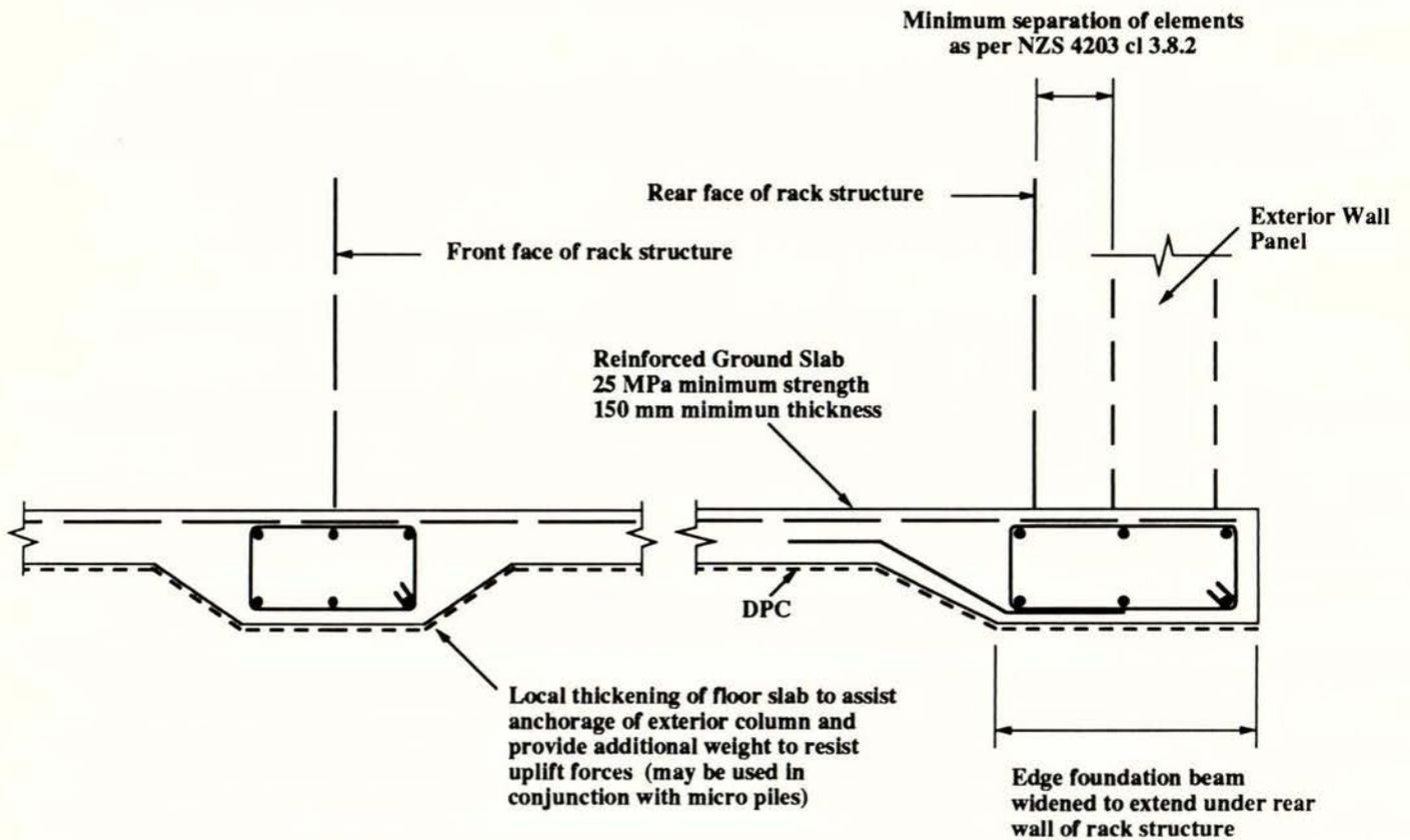
**Note:** Cast ground slab integral with foundation beams to provide increased resistance against uplift
