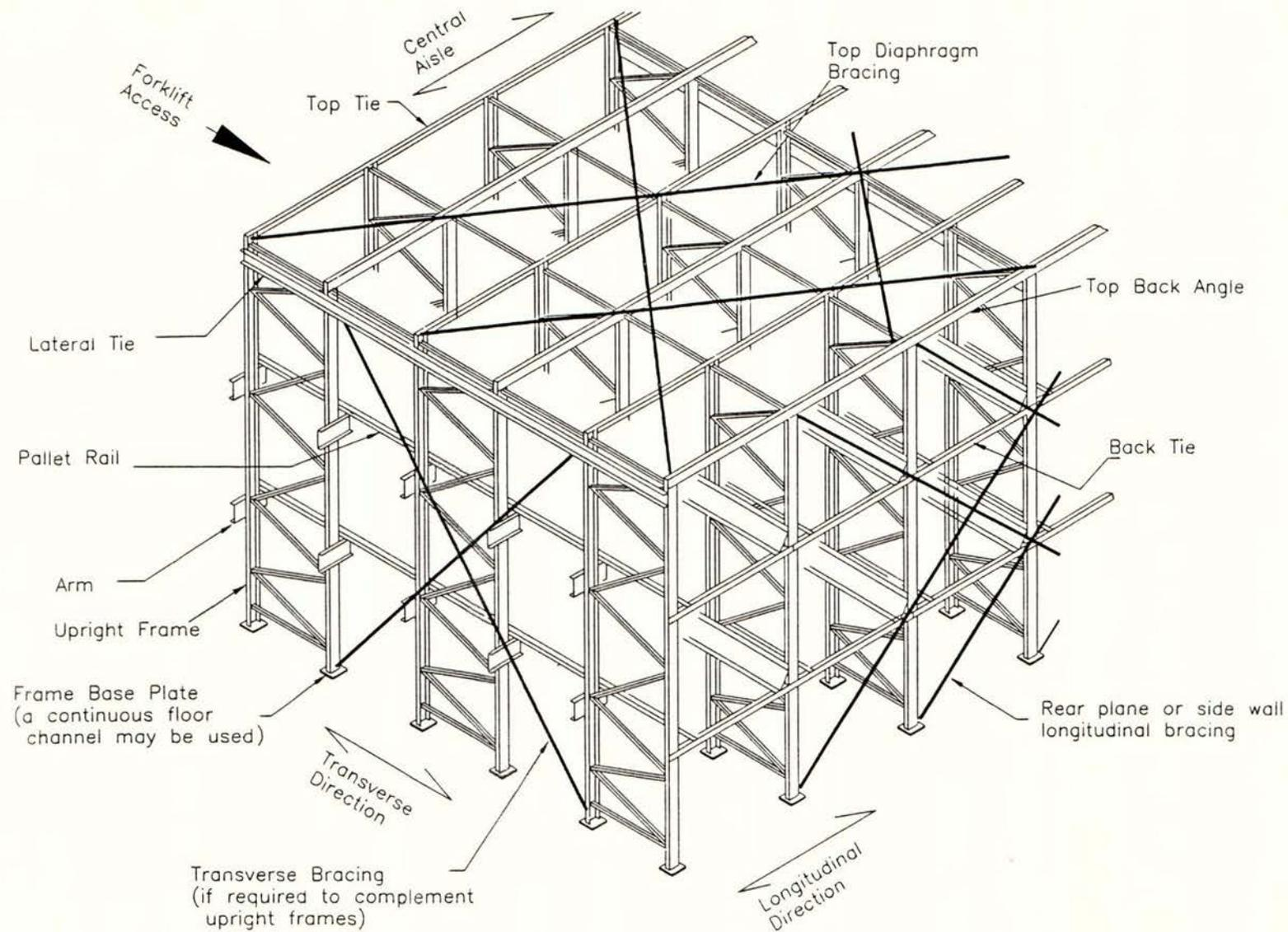
Fig 1.1 Typical Drive-in Pallet Racking System With Additional Seismic Bracing
