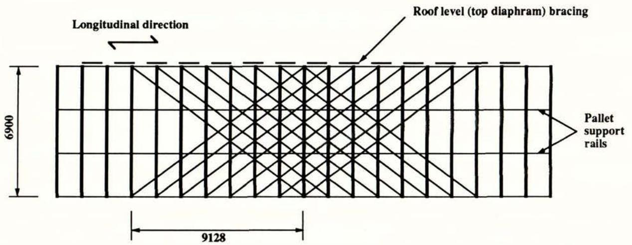
**Rear Elevation - Showing Rear Plane (Side Wall) Longitudinal Bracing**
