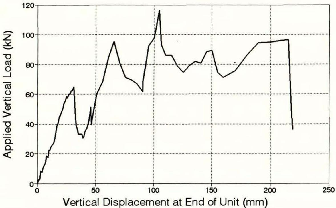
Fig. 6.7 Applied Vertical Load Versus Vertical Displacement at End of Unit Measured During the Second Stage of Test B on Connection Type 1
