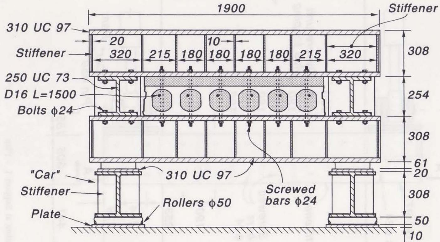
Fig. 3.2c Hinge Mechanism at Support 1. - Section A-A
