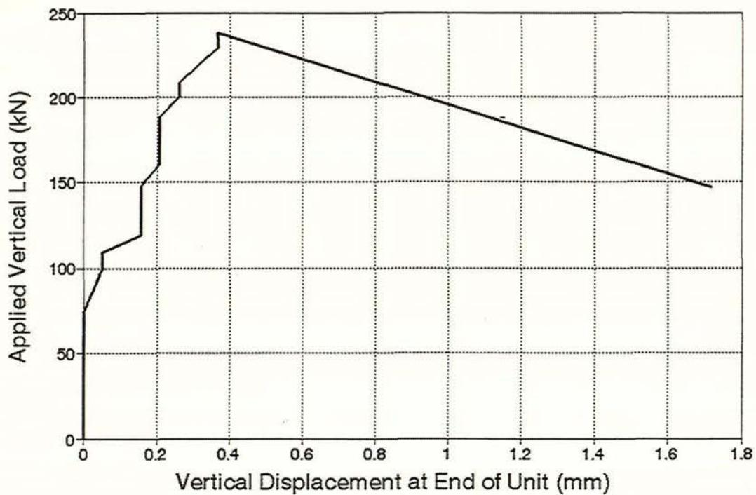
Fig. 5.6 Applied Vertical Load Versus Vertical Displacement at the End of Unit Measured During Test A on Connection Type 2
