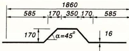
(b) Connection Type 2: Two deformed bars, 16mm diameter, Grade 300
