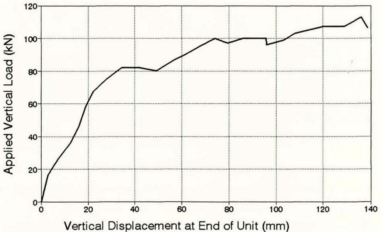
Fig. 6.12 Applied Vertical Load Versus Vertical Displacement at End of Unit Measured During the Second Stage of Test B on Connection Type 3
