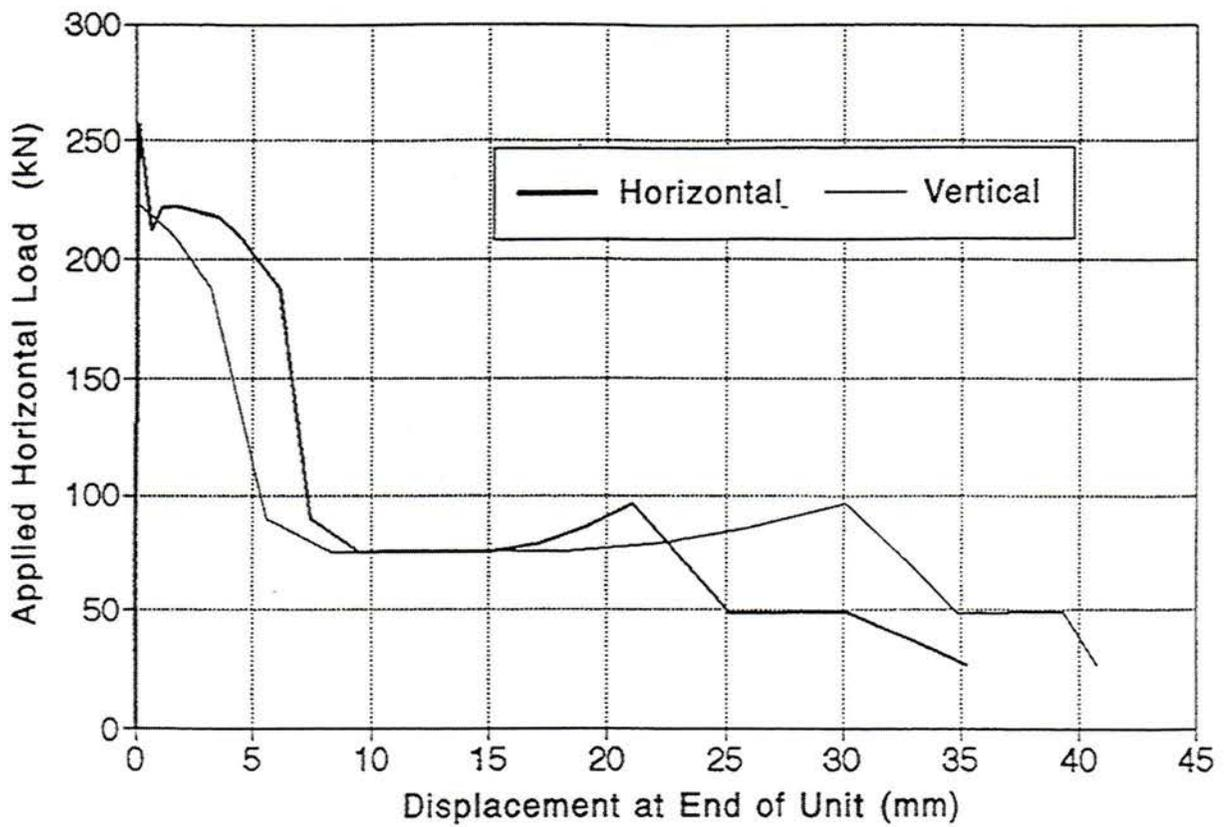
Fig. 6.9 Applied Horizontal Load Versus Horizontal and Vertical Displacements at End of Unit Measured During the First Stage of Test B on Connection Type 2
