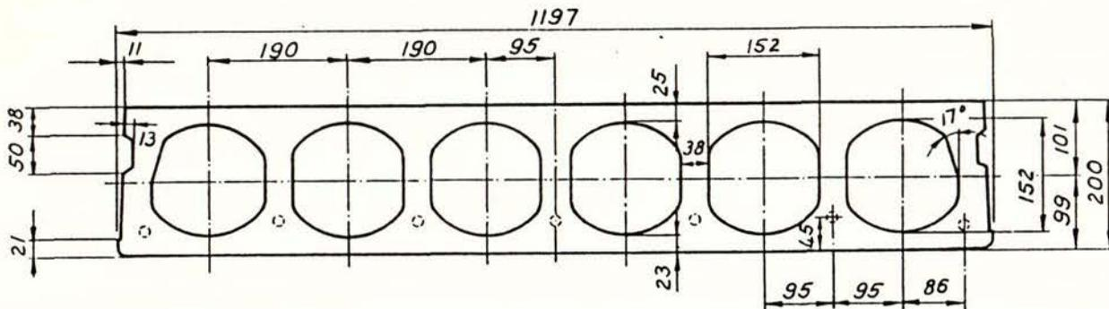
Fig. 3.8 Dimensions of Dy-core Used in the Tests
