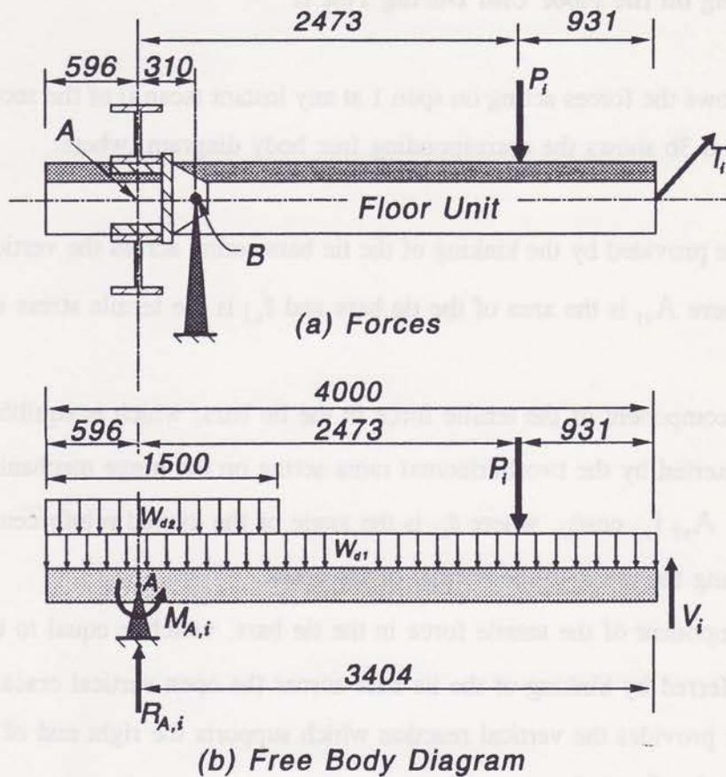
Fig. 6.3 Forces Acting in Span 1 During Second Stage of Test B
