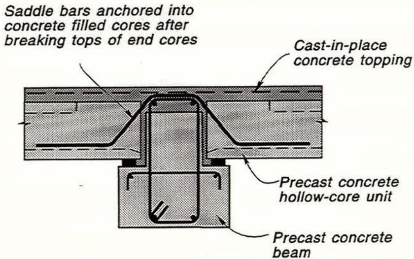
Fig. 1.3 Saddle Bars for Precast Hollow-Core Units According to the New Zealand Guidelines [1]
