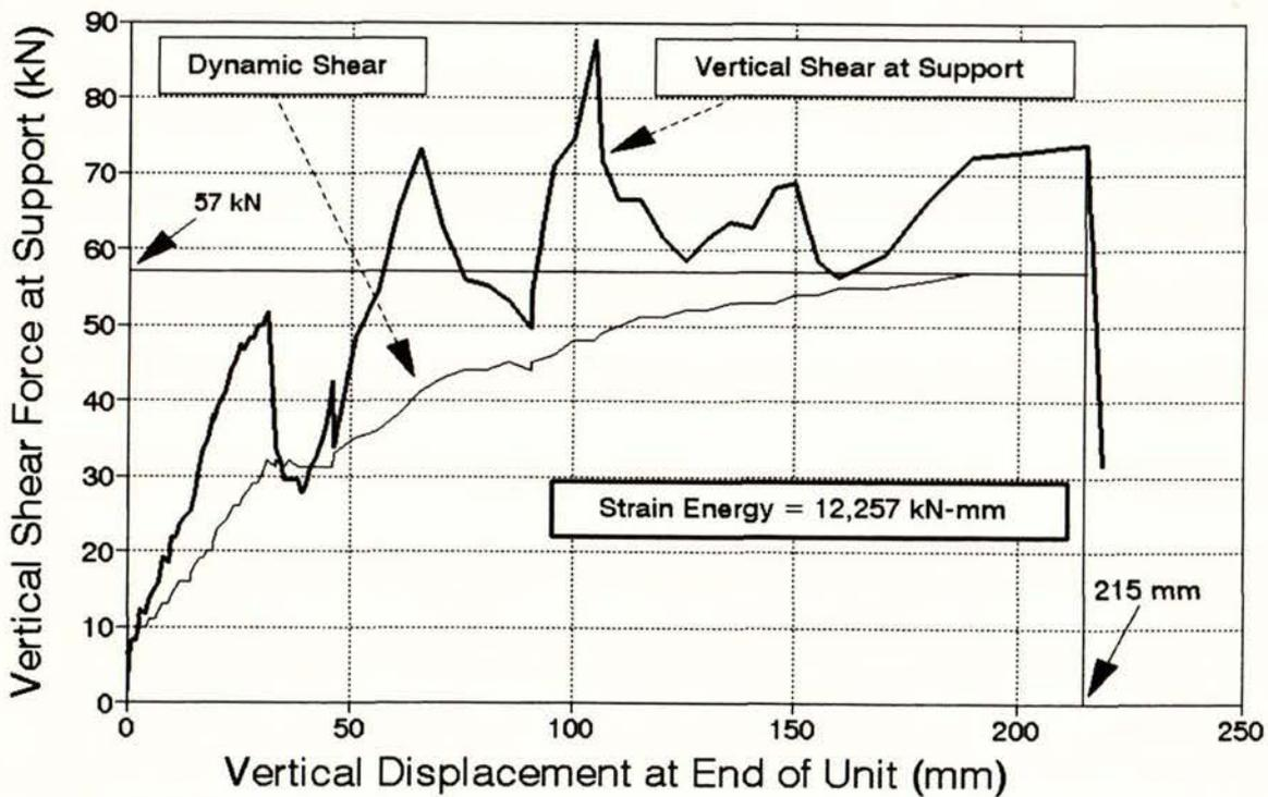
Fig. 6.8 Vertical Shear Force at the Support and Equivalent Dynamic Shear Capacity of the Connection Versus Vertical Displacement at the End of Unit Measured During the Second Stage of Test B on Connection Type 1
