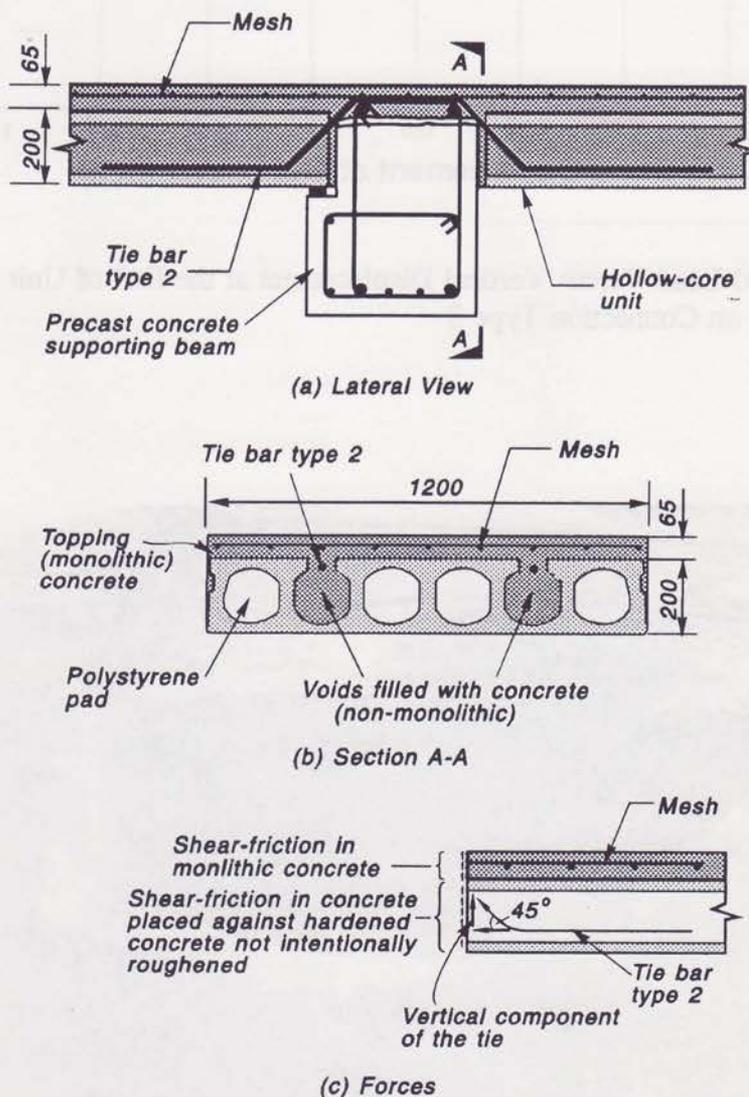
Fig. 5.8 Transfer of End Reaction by Shear Friction During Test A of Connection Type 2
