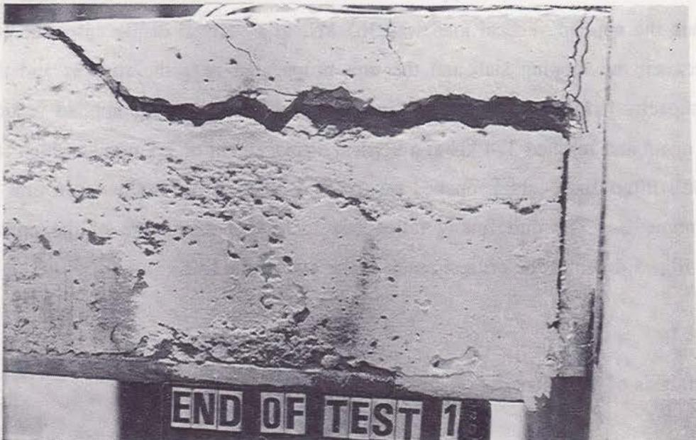
Fig. 5.4 Connection Type 1 at End of Test A
