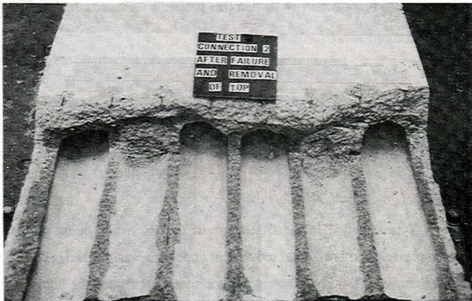
Fig. 6.10 At the End of Test B on Connection Type 2
