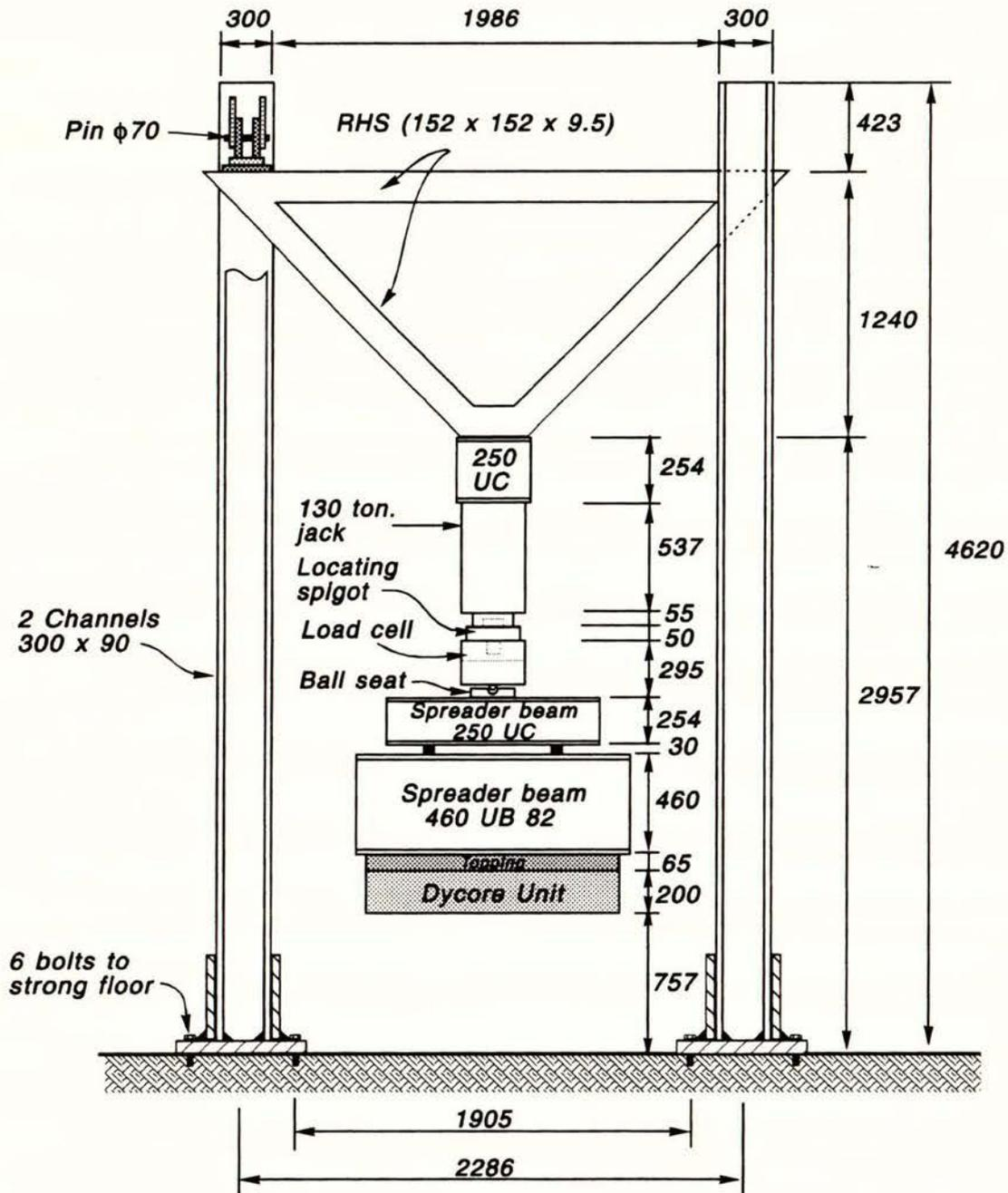
Fig. 3.11 Vertical Loading System of Test A and B
