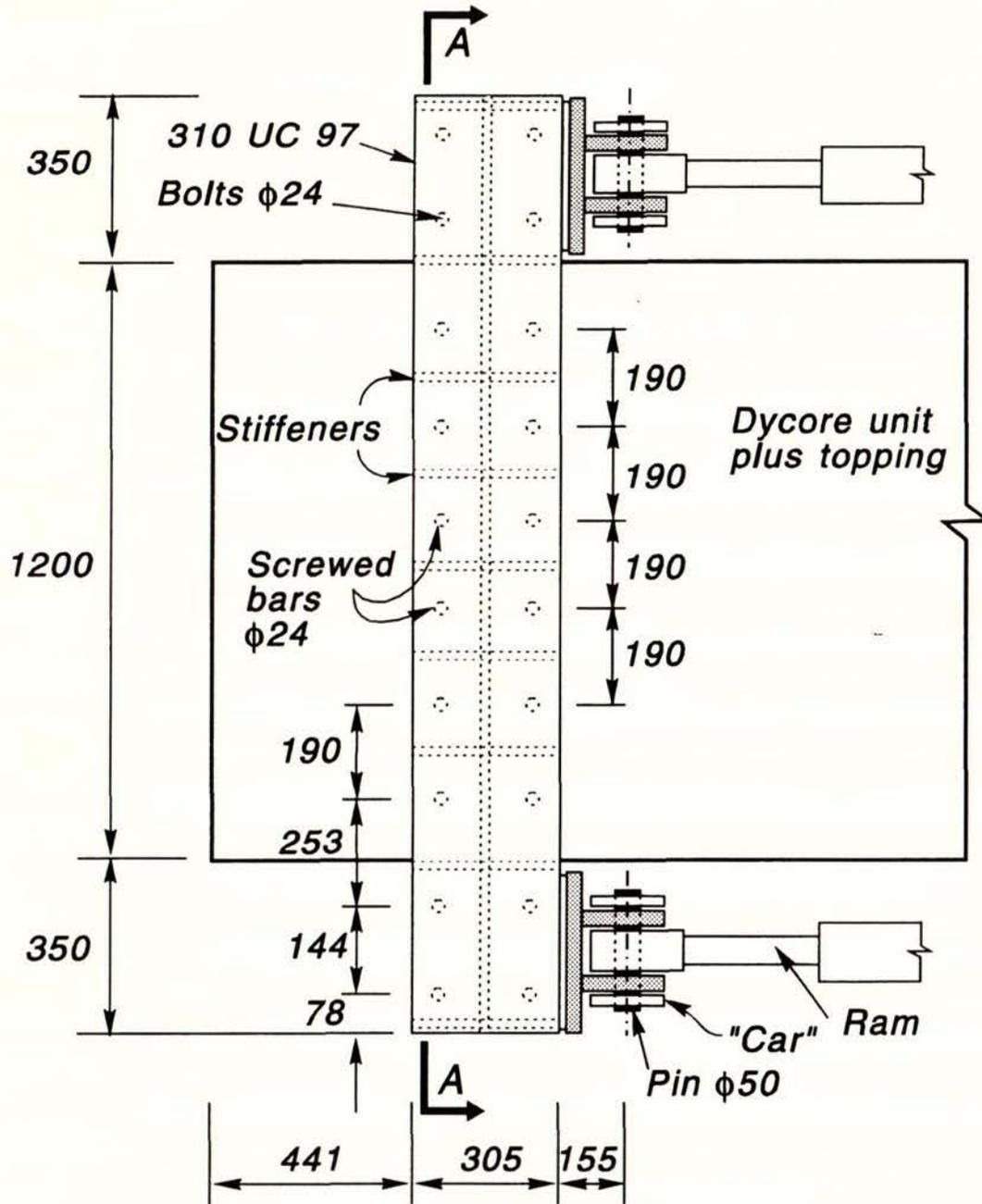
Fig. 3.2b Hinge Mechanism at Support 1. - Plan
