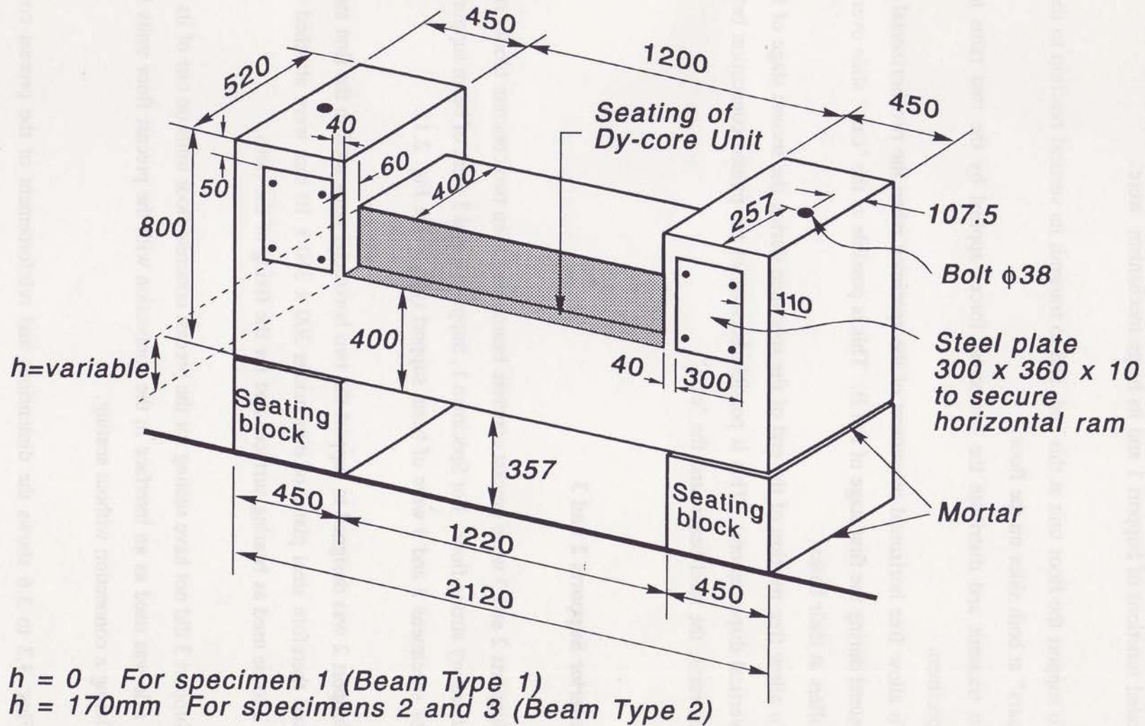
Fig. 3.3 Dimensions of Precast Concrete Beam Used as Support 2.
