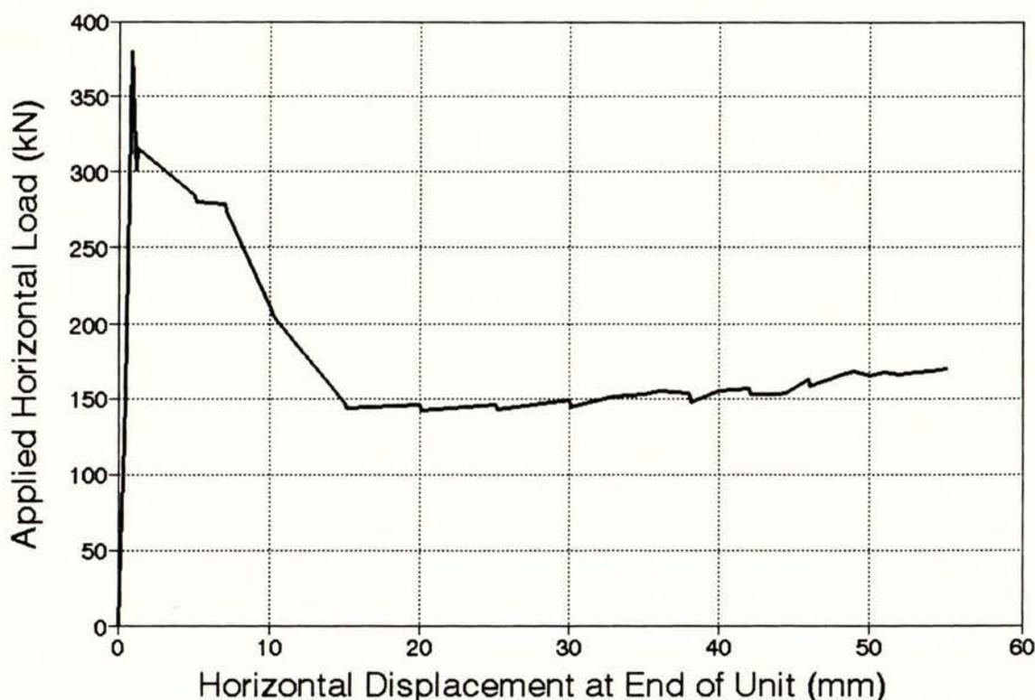
Fig. 6.4 Applied Horizontal Load Versus Horizontal Displacement at the End of Unit Measured During First Stage of Test B on Connection Type 1
