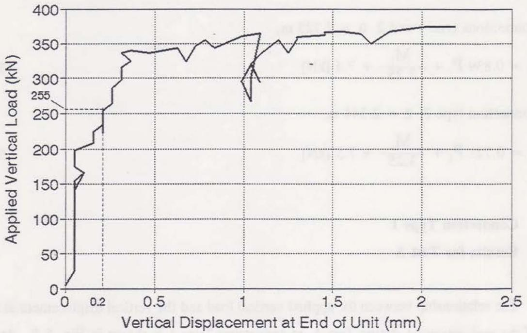
Fig. 5.3 Applied Vertical Load Versus Vertical Displacement at the End of Unit Measured During Test A on Connection Type 1
