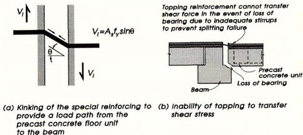
Fig. 1.1 Kinking of Reinforcement and Possible Failure of Topping if Bearing of Precast Unit is Lost According to the New Zealand Guidelines [1]
