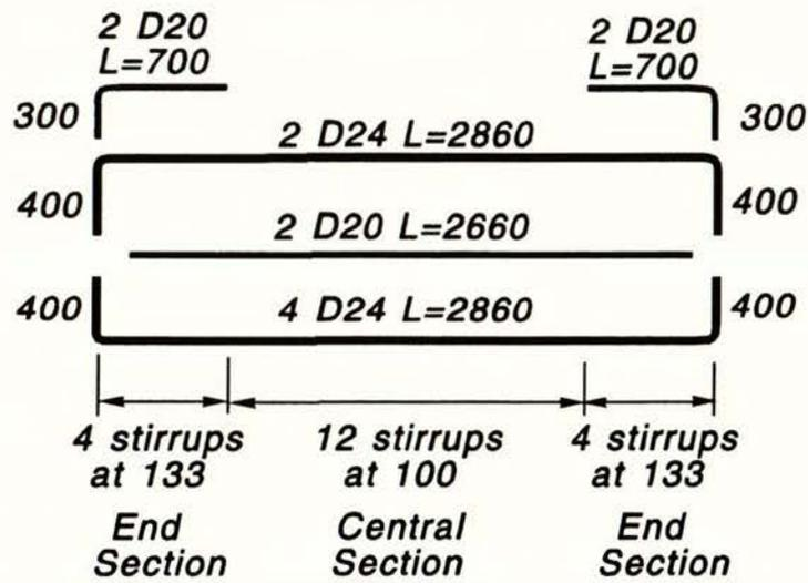
(a) Longitudinal Reinforcement and Stirrups
