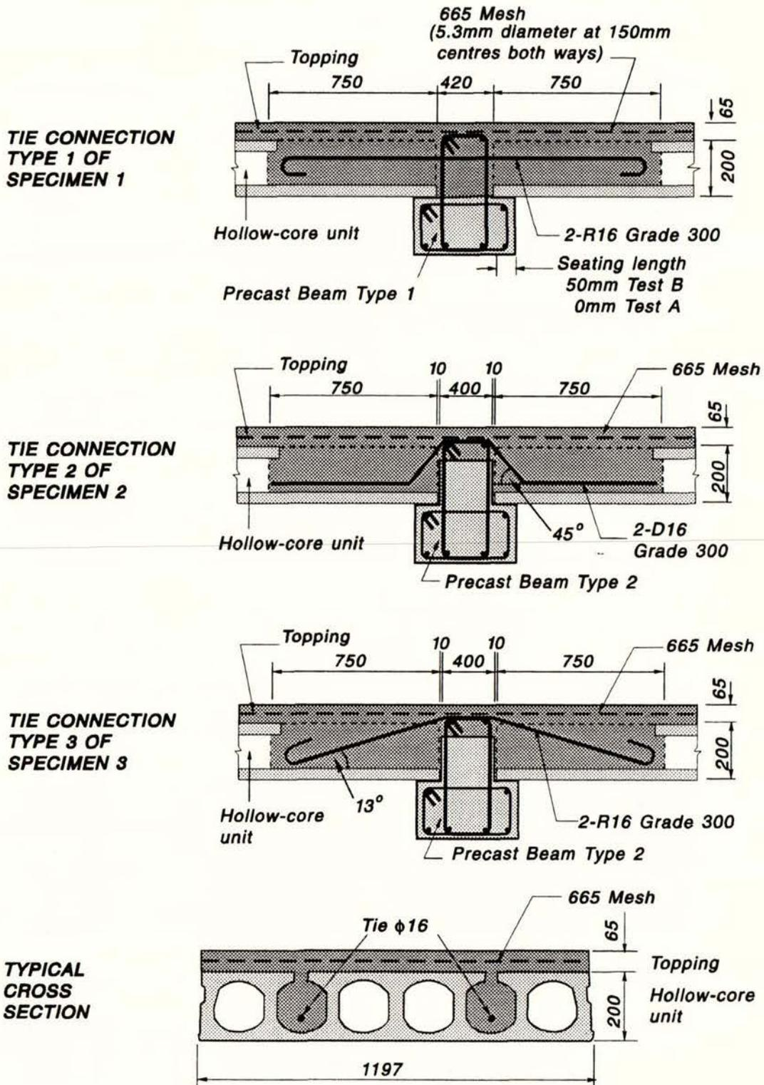
Fig. 2.2 Details of the Tie Connections Tested
