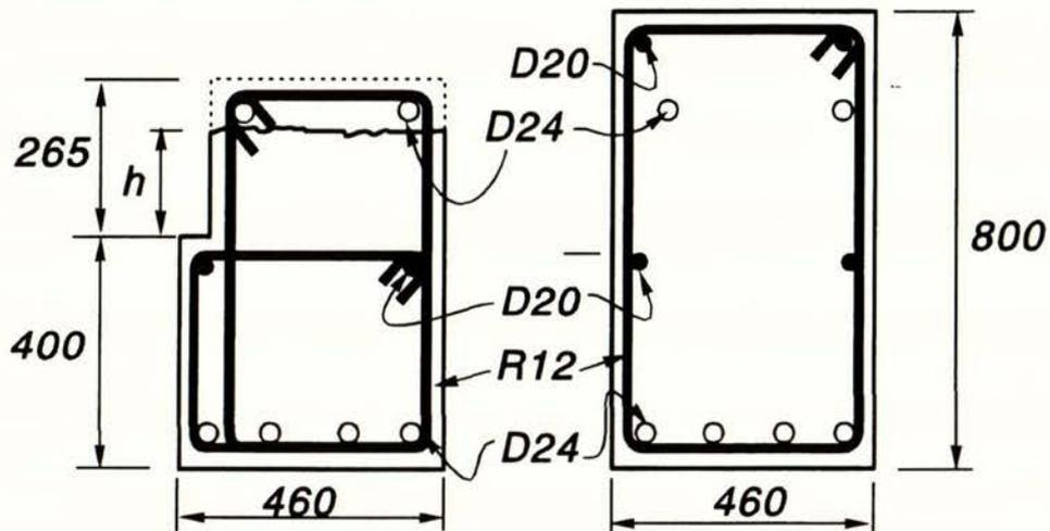
Beam Central Section      Beam End Section
