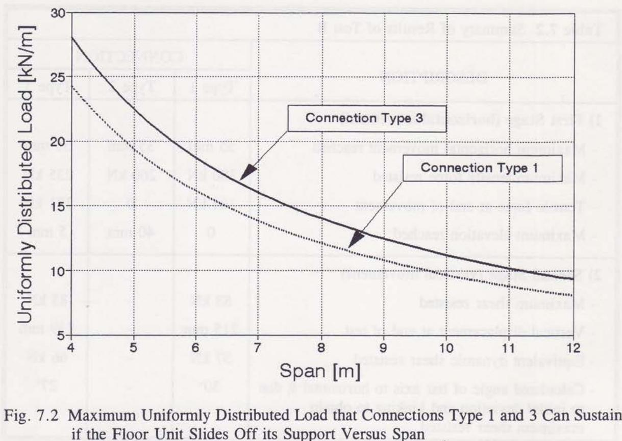
Fig. 7.2 Maximum Uniformly Distributed Load that Connections Type 1 and 3 Can Sustain if the Floor Unit Slides Off its Support Versus Span
