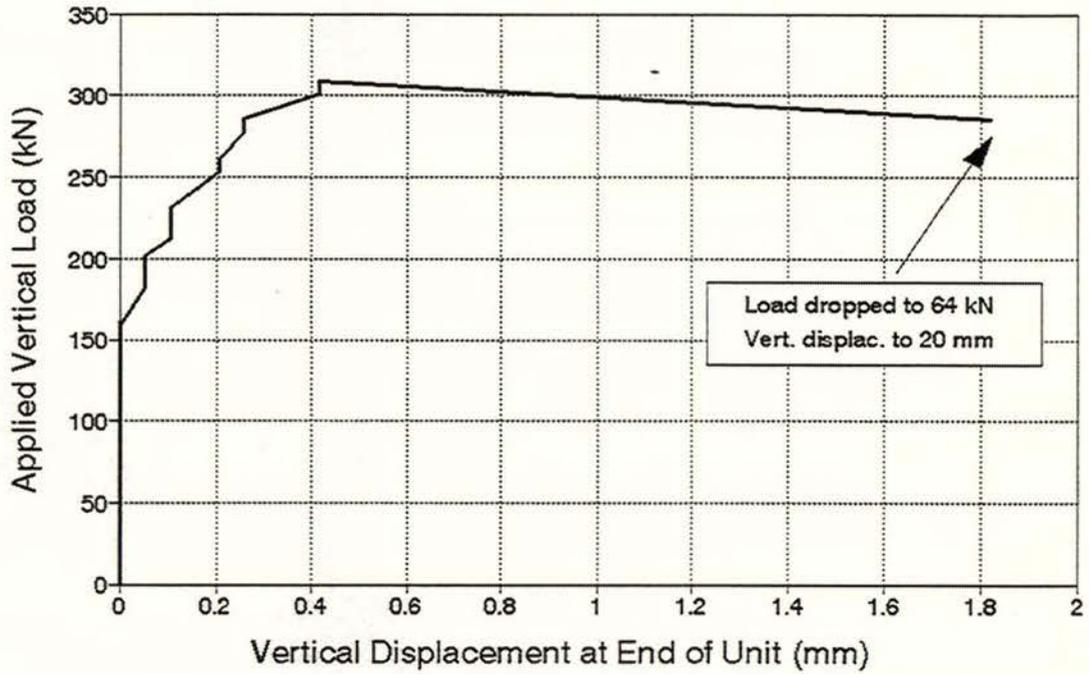
Fig. 5.9 Applied Vertical Load Versus Vertical Displacement at the End of Unit Measured During Test A on Connection Type 3
