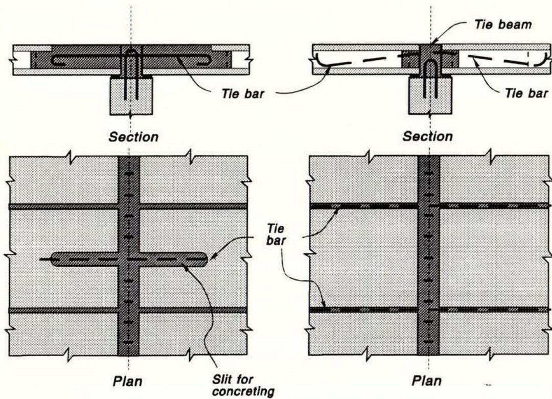
Fig. 1.4 Details of Tie or Continuity Reinforcement Suggested by the FIP [2]
