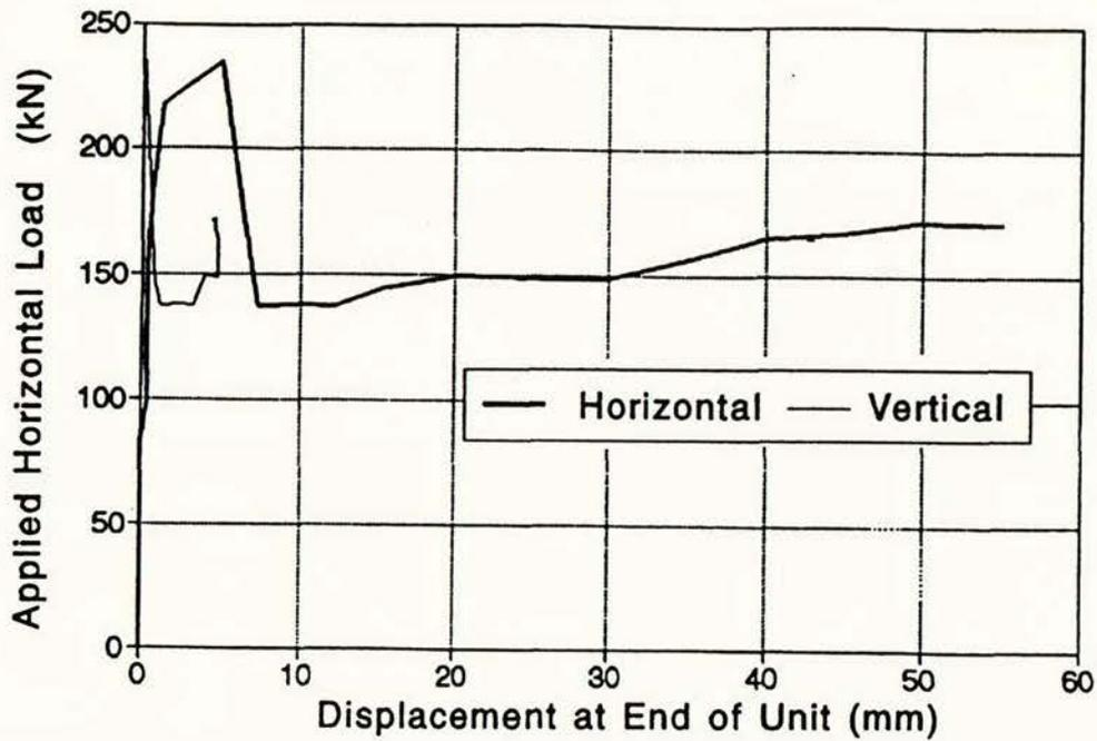
Fig. 6.11 Applied Horizontal Load Versus Horizontal and Vertical Displacements at End of Unit Measured During the First Stage of Test B on Connection Type 3
