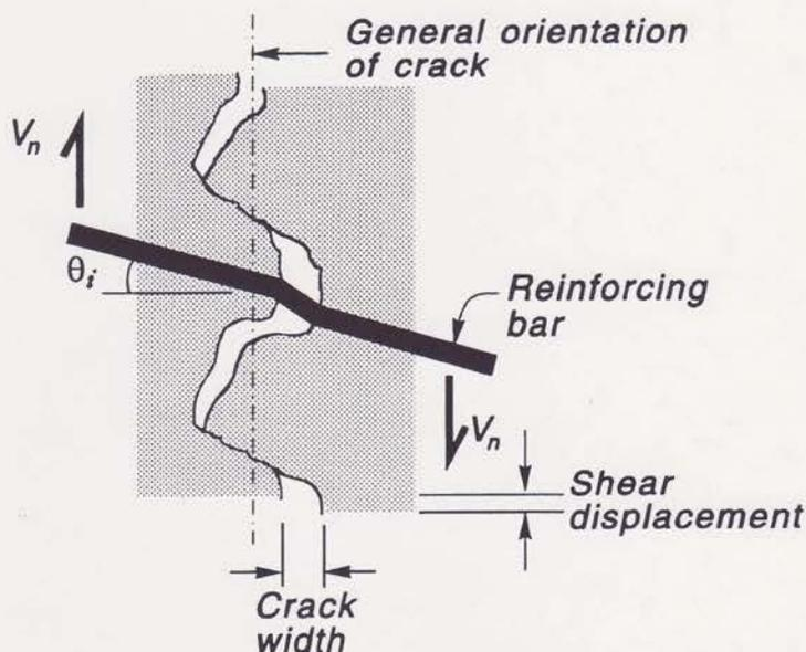
Fig. 5.1 Shear Transferred by Interface Friction Across a Narrow Crack
