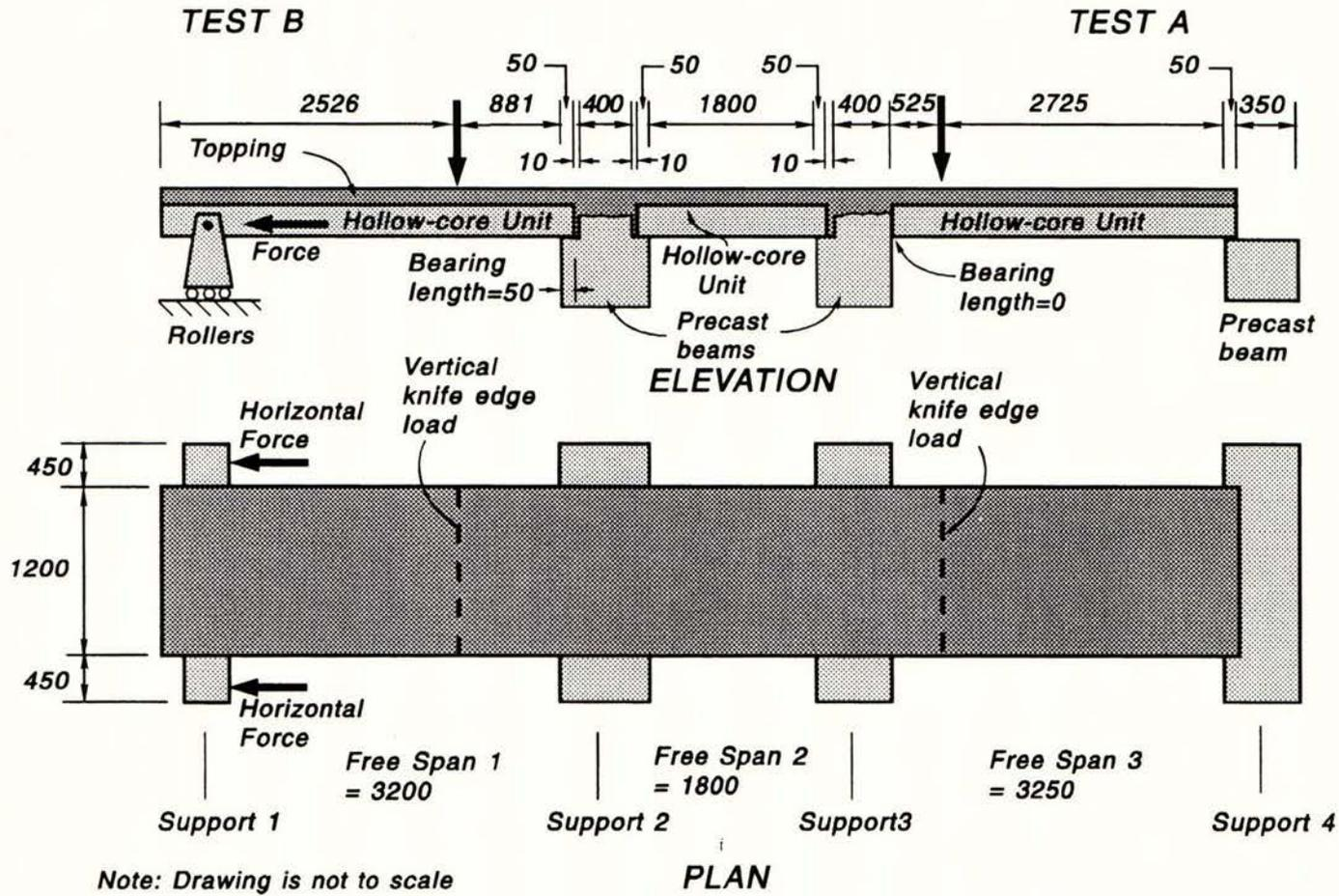
Fig. 3.1 Dimensions and Test Set-Up of Specimens.
