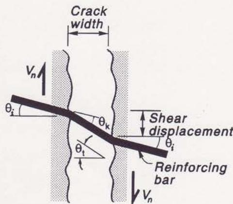
Fig. 6.1 Shear Transferred by Kinking of Reinforcement Across a Wide Crack
