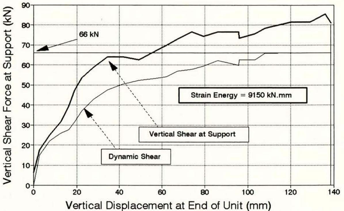
Fig. 6.14 Vertical Shear Force at the Support and Equivalent Dynamic Shear Capacity of the Connection Versus Vertical Displacement at the End of Unit Measured During the Second Stage of Test B on Connection Type 3
