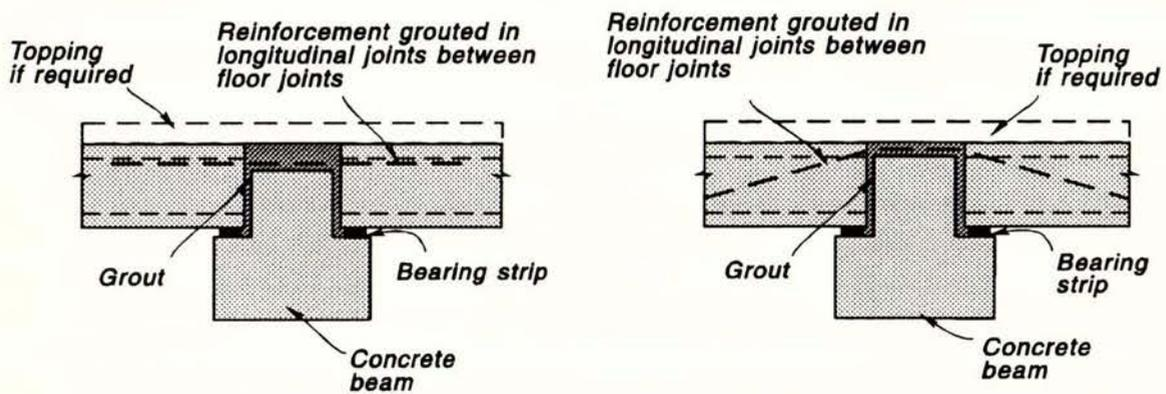
Fig. 1.5 Details of Tie or Continuity Reinforcement Suggested by the PCI [3]
