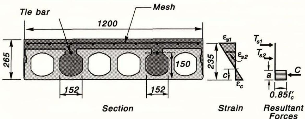
Fig. 5.5 Section at Flexural Strength on Test A of Connection Type 1
