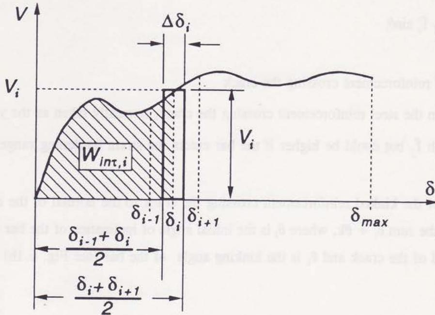
Fig. 6.2 Typical Relationship Between Vertical Shear Force at the Support and the Vertical Displacement at End of Unit
