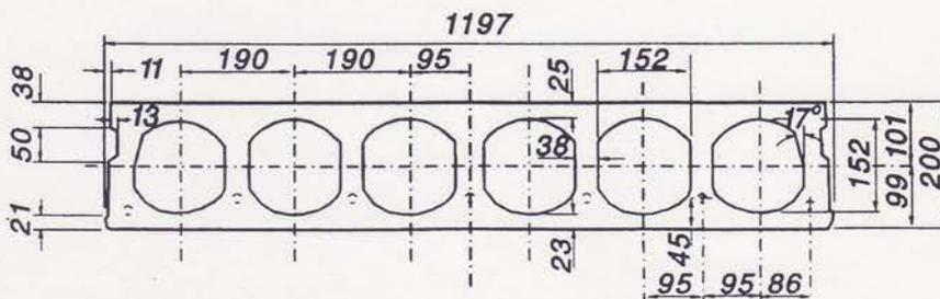
Fig. A Dimensions of the Precast Concrete Hollow-Core Unit Used in the Tests
