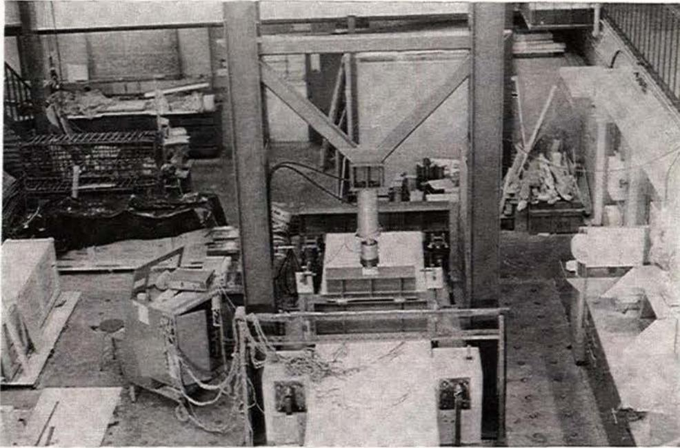
Fig. 3.13 Vertical Loading System in Position for Test B
