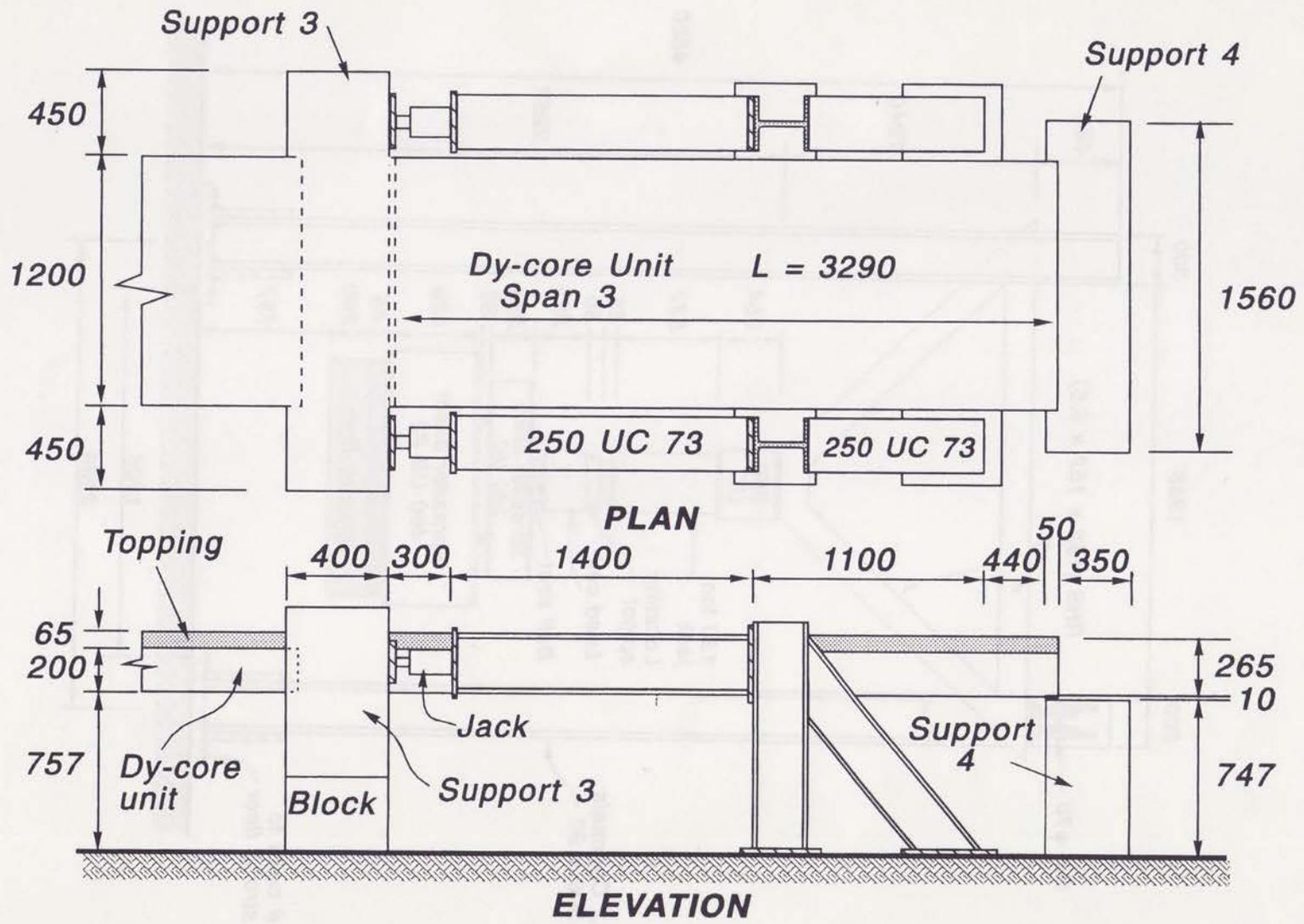
Fig. 3.12 Horizontal Restraint System of Support 3
