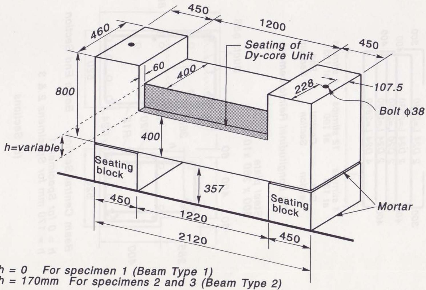
Fig. 3.5 Dimensions of Precast Concrete Beam Used as Support 3.
