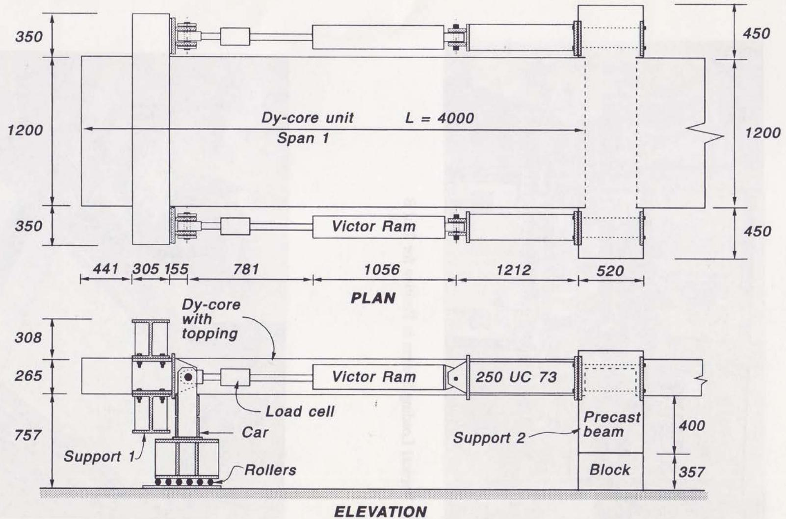
Fig. 3.15 Horizontal Loading System of Test B
