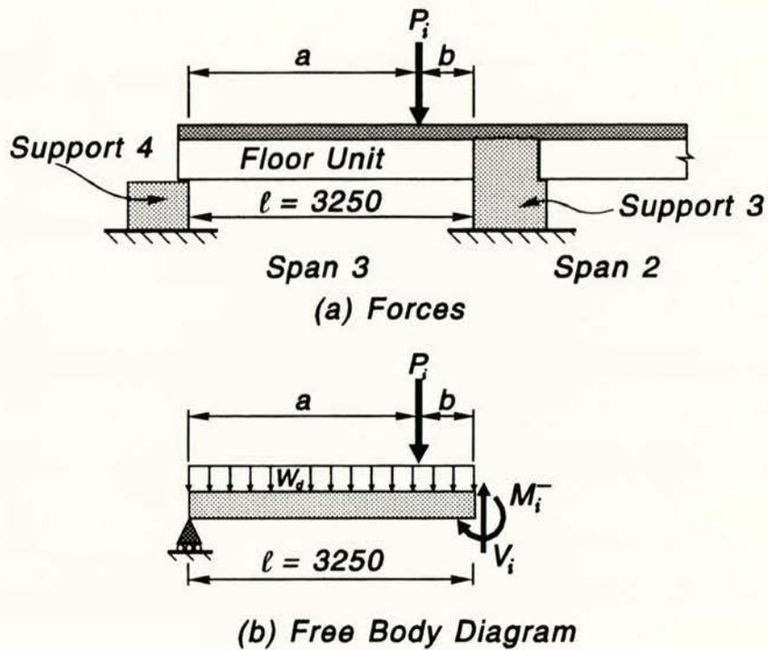
Fig. 5.2 Forces Acting in Span 3 During Test A
