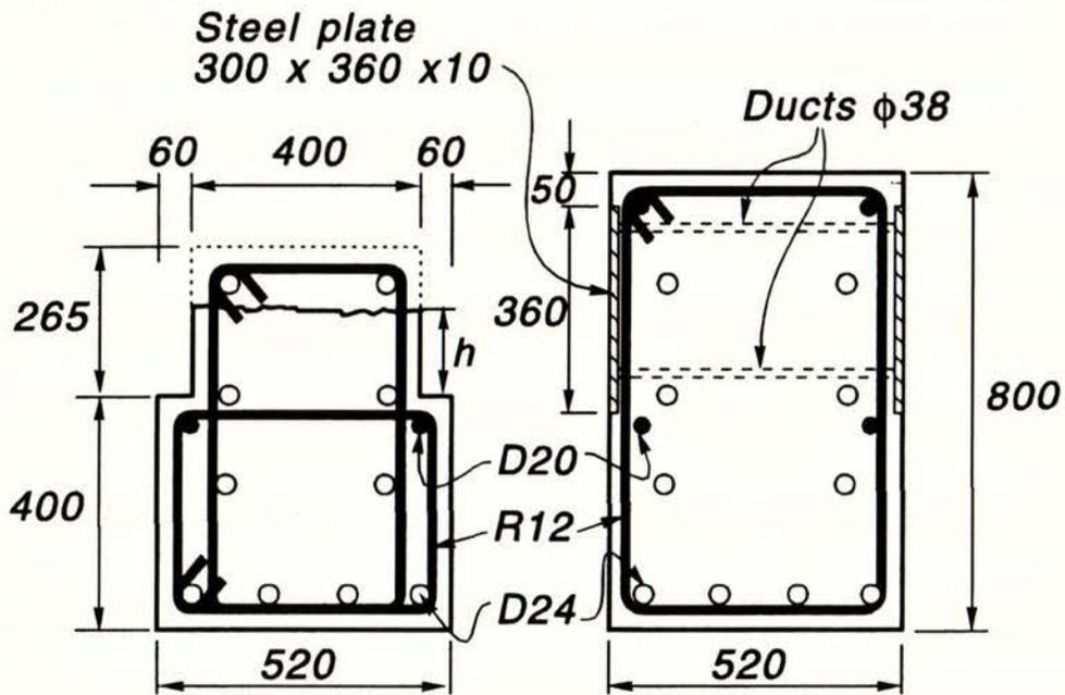
Beam Central Section      Beam End Section
