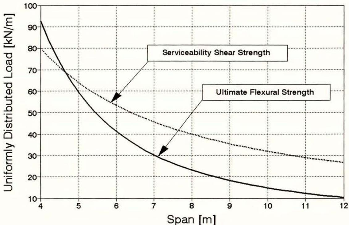
Fig. 7.1 Uniformly Distributed Load Versus Span at Serviceability Shear Strength and Ultimate Flexural Strength
