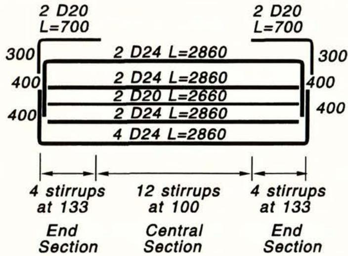
(a) Longitudinal Reinforcement
