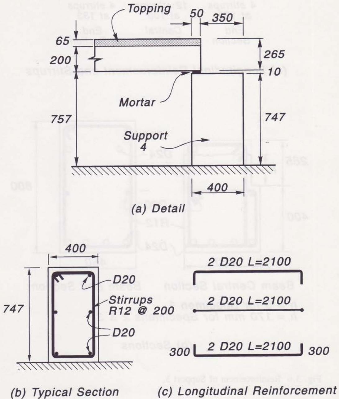
Fig. 3.7 Dimensions and Reinforcement of Support 4
