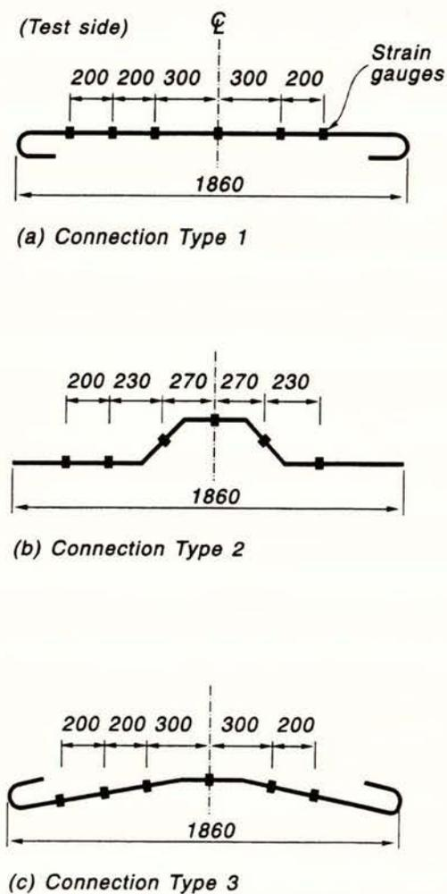
Fig. 3.16 Position of the Electrical Resistance Strain Gauges on the Tie Bars
