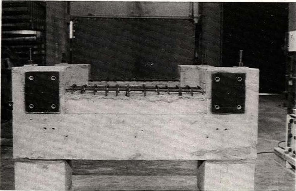
Fig. 3.9b Supports Plastered in Their Position
