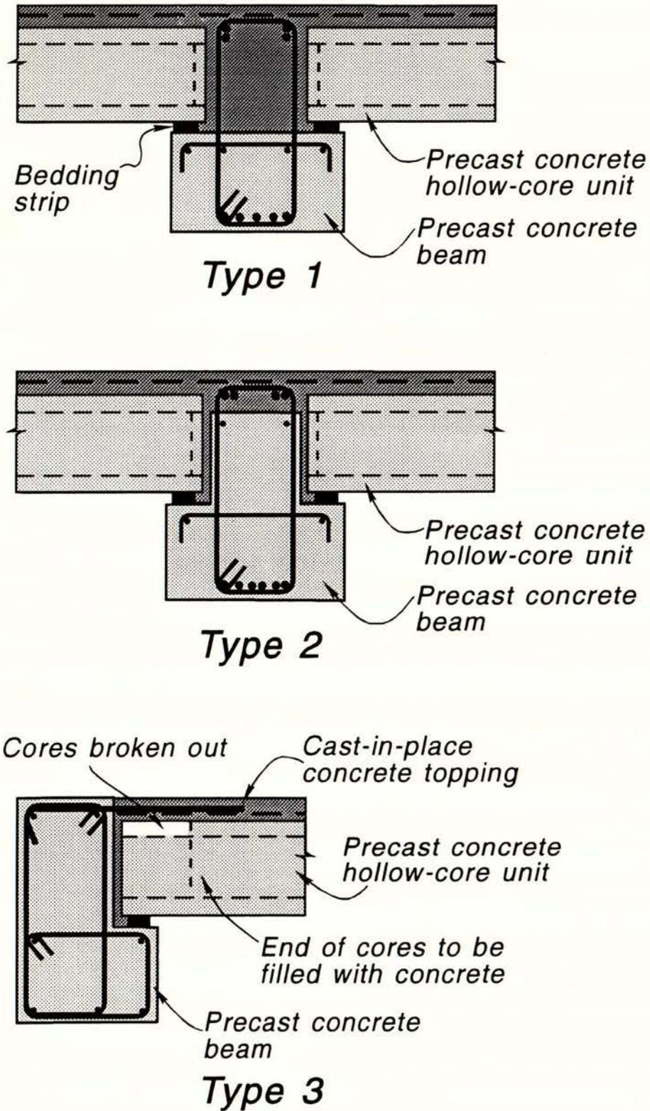
Fig. 2.1 Types of Support of Precast Concrete Hollow-Core Floor Units by Precast Concrete Beams According to the New Zealand Guidelines [1]
