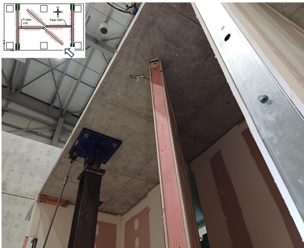
Figure 2.69. Walls from North-East direction after motion 18 - 3 % inter-storey drift
