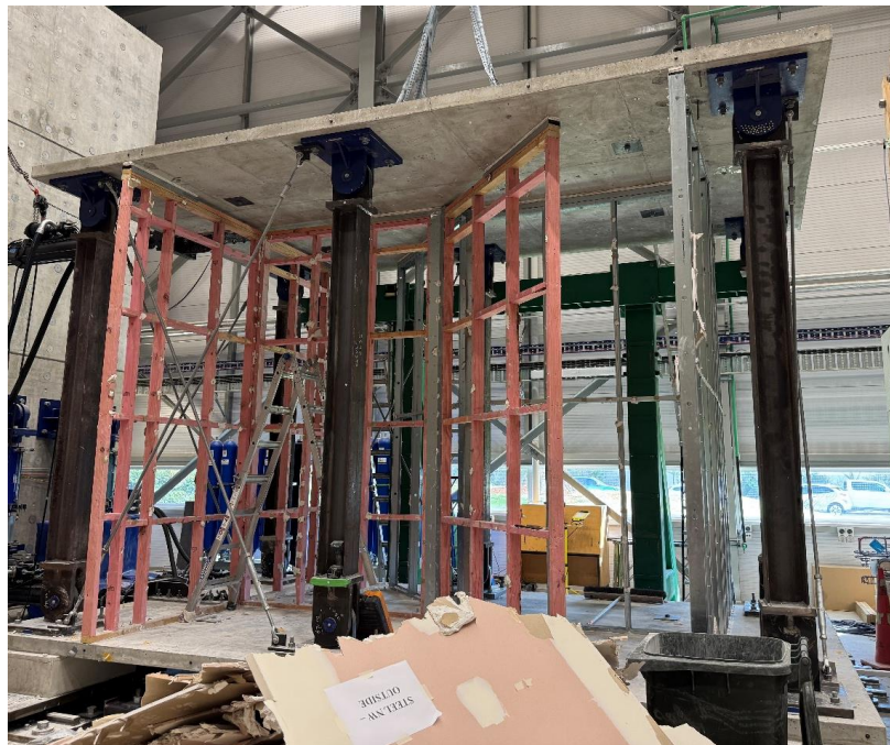
Figure 2.71. Photo of wall frames after motion 18 - 3 % inter-storey drift (Southeast elevation)
