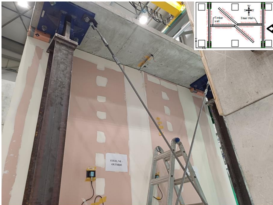
Figure 2.57. Steel NE Outside wall after motion 18 - 3 % inter-storey drift
