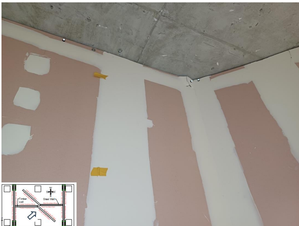
Figure 2.66. Timber Southeast Inside wall after motion 18 - 3 % inter-storey drift
