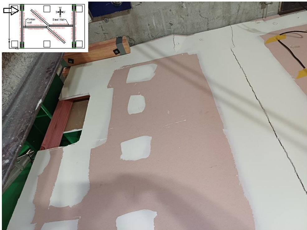
Figure 2.62. Timber South-West Inside wall after motion 18 - 3 % inter-storey drift
