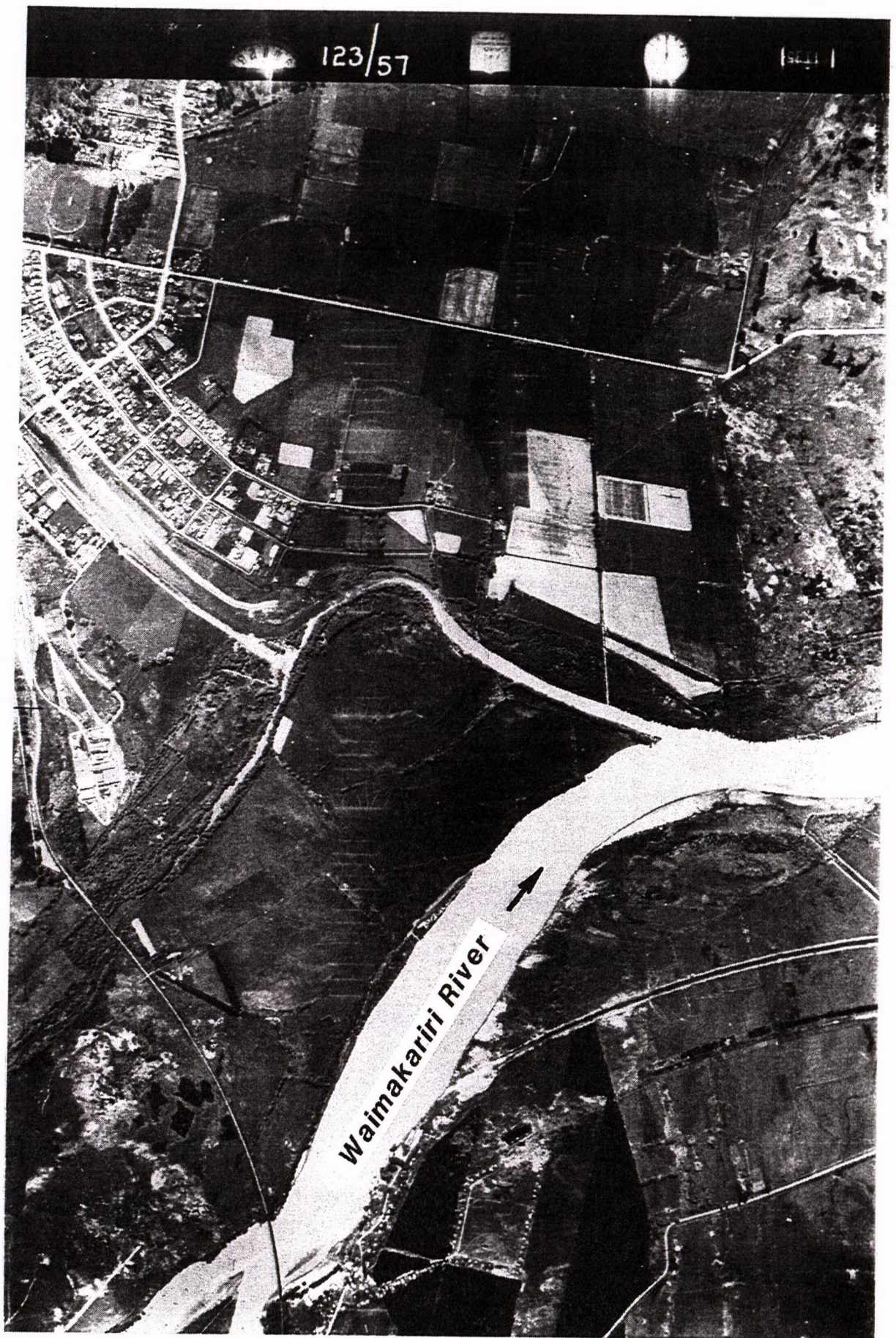
Figure 2 A 1941 aerial photograph of north east Kaiapoi. The Kaiapoi River flows into the Waimakariri River, seen in the lower right of the photograph. Note the semi-circular feature north of Cass Street near the centre of the photo, denoting a former meander loop of the Waimakariri. Several other, less prominent, meanders are seen in this photograph. (Photo: NZ Aerial Mapping)
