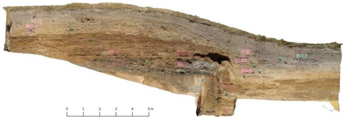
Figure 8: South (only) wall of the Branch Creek trench, showing interpreted log (top) and orthophoto mosaic (bottom). The actual NW Cardrona Fault is shown by the red lines. Source is van den Berg (2020).
