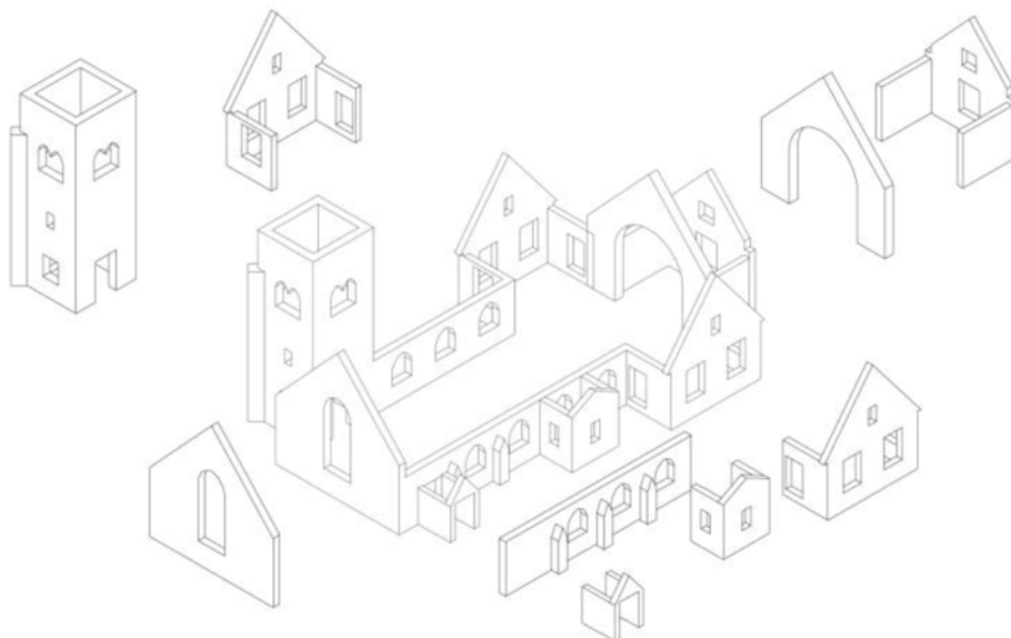
Figure A3.1 Composition of the church in the macroelements.
