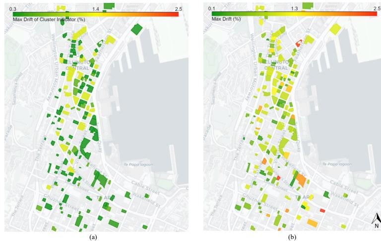
Figure 3. Drift maps using two methods; (a) Method One: drifts driven from indicator buildings (b) Method Two: drifts driven from linear regression response model.
