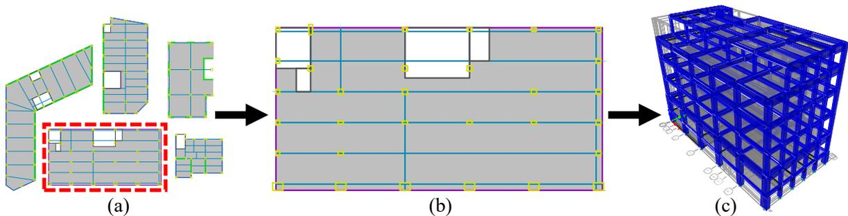
Figure 2. Cluster 0 (a): top five ranked buildings floor plans, (b): the selected indicator building floor plan, and (c): the rendered sketch of ETABS model for indicator building.
