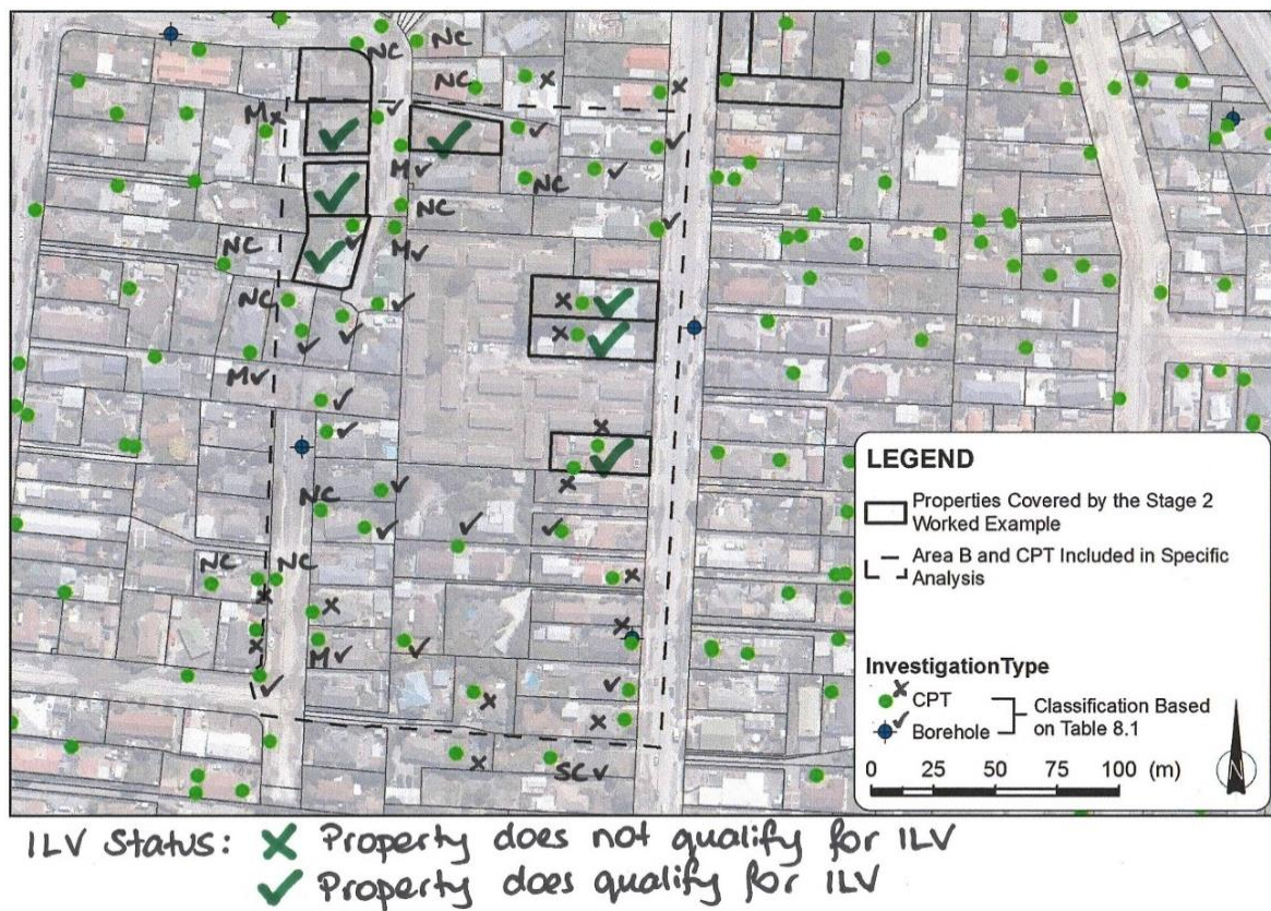
Figure L3.5: The location and classification of the CPT and boreholes and the ILV qualification of the properties for the Stage 2 manual assessment pack in Area B.
